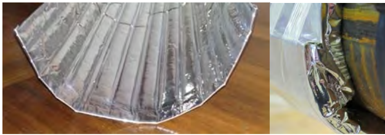
Figure 2. a) Surface of a cylindrical VIP b) overlap mounting of VIP
