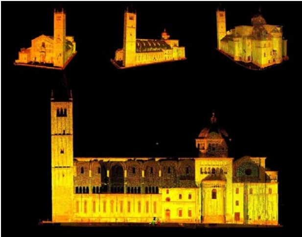
Figure 4_The complete point cloud after registration.
