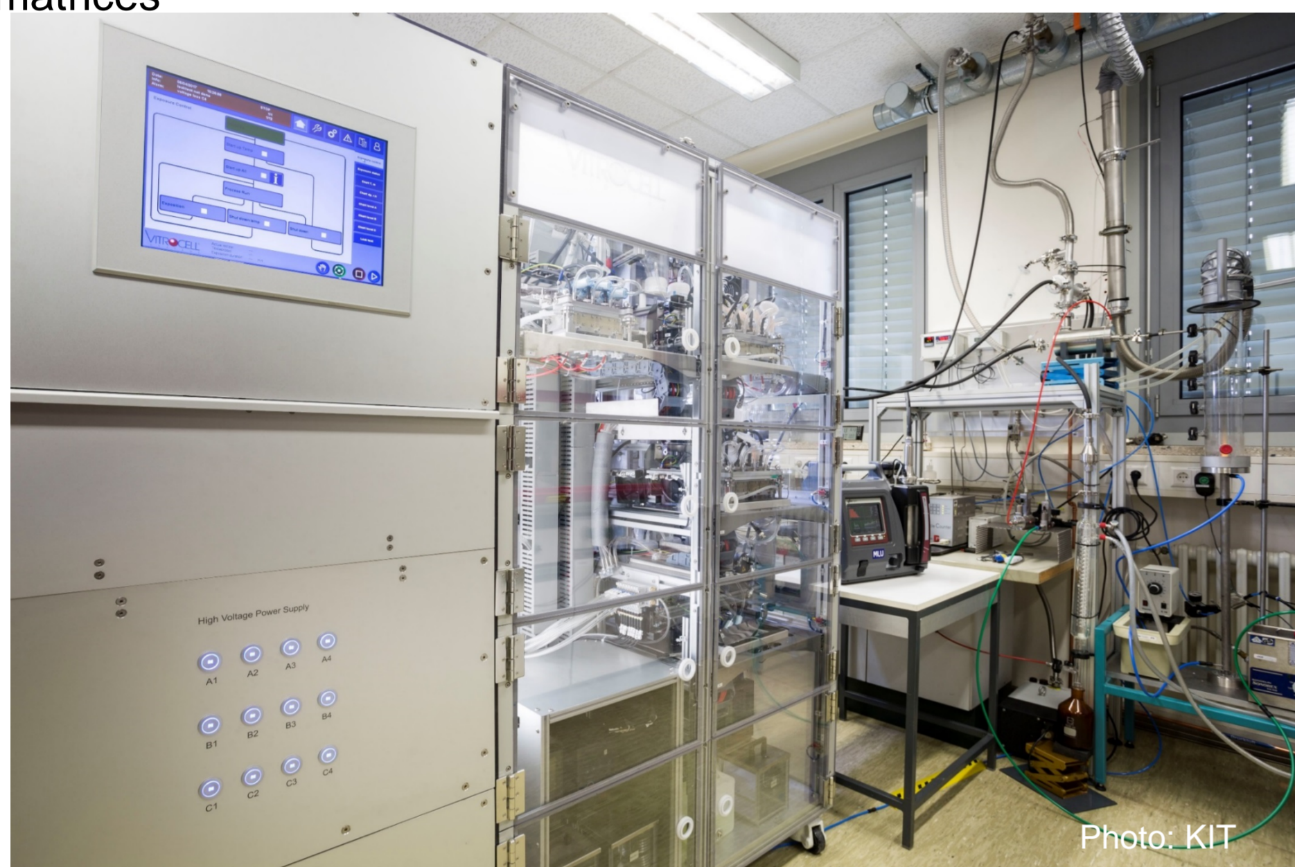
Laboratory setup with Vitrocell® Automated Exposure Station, ELPI and tube burner.
