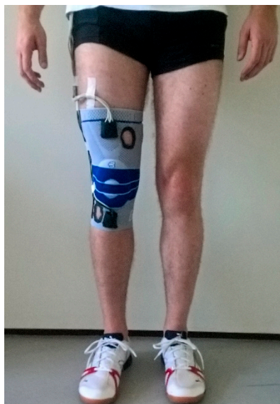
Figure 1. Placement of inertial measurement units (IMUs) used in the study. The IMUs were positioned in the two black patch pockets at the upper and lower frontal end of the sleeve.
