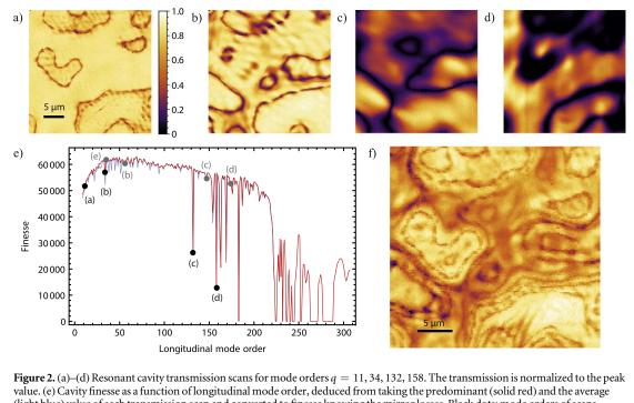
(light blue) value of each transmission scan and converted to finesse knowing the mirror losses. Black dots: mode orders of scans (a)–(d). Gray dots: mode orders of scans (b)–(e) in figure 6. (f) Overlay of transmission scans of longitudinal mode orders q = 11, 12, 14, 16, 22, 24, 28, 38 yielding a consistent isocontour map. Color scale: see (a).
