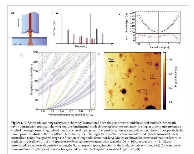
shape affect the mode structure. It has been shown that such imperfect mirror shape and finite mirror size can lead to loss, mode deformation, and shifted resonance frequencies at particular mirror separations [17]. The behavior is explained by resonant coupling between different transverse modes of the cavity and modedependent diffraction loss. The effects can be quantified by a model based on resonant state expansion [31] that takes the measured mirror profile into account.
