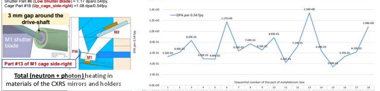
Maximum values found in the following Mo components: Cage part #13 (Low_cage_side-right) equalled 1.34 dpa per 0.54 fpy. Shutter Part #6 (Low Shutter Blade) = 1.17 dpa/0.54fpy. Cage Part #18 (Up_cage_side-right) = 1.06 dpa/0.54fpy.
