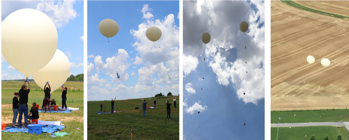
Figure 4. A time-lapse of fill and launch procedures from national dry run. The first three images taken from the ground while the final image take from a fixed-wing aircraft.
