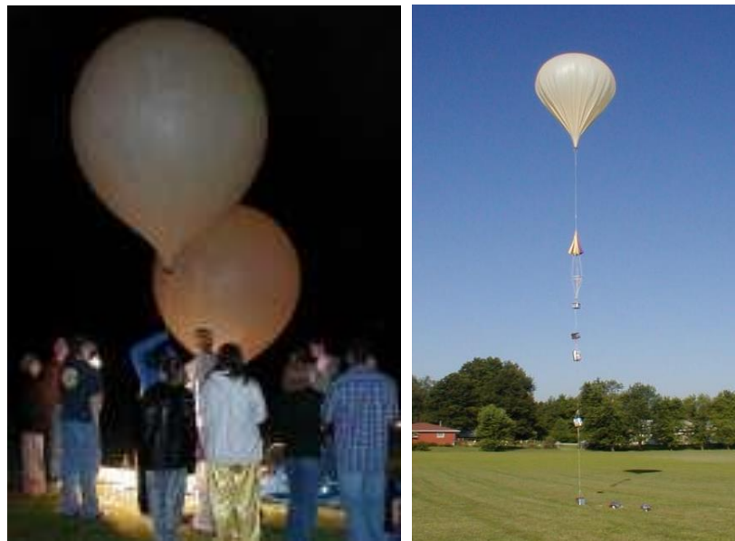
Fig. 7 Secondary balloon nighttime astronomy launch and resulting landing configuration with just the secondary still inflated. Note the stretch marks on the secondary balloon after it returned from high altitude flight. The balloon was actually successfully flown on another flight.
