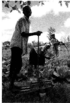
Foot-pump irrigation system designed by KickStart and made available to farmers in Kenya. Public Domain
