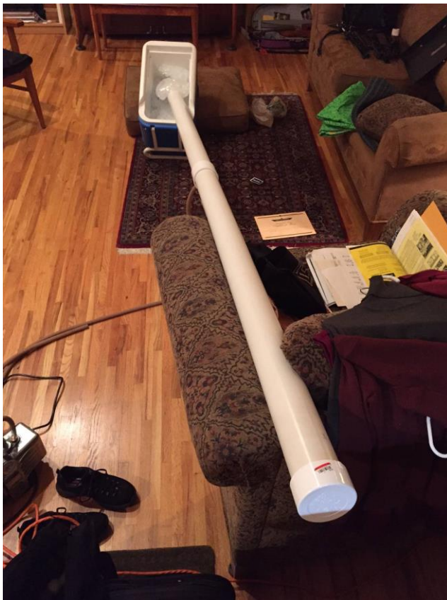
Figure 5(b) – PCV pipe set-up for reduced-pressure test
