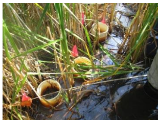
Figure 1.2: Example of chamber installation, pictured here is a Typha control plot. Photo credit: Olivia Johnson.
