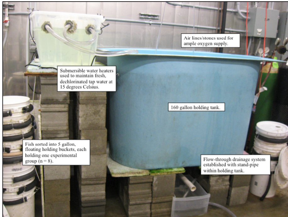
Figure A. Indoor flow-through tank where fish were held between swimming challenges, maintained within a 15 degrees Celsius cold room.
