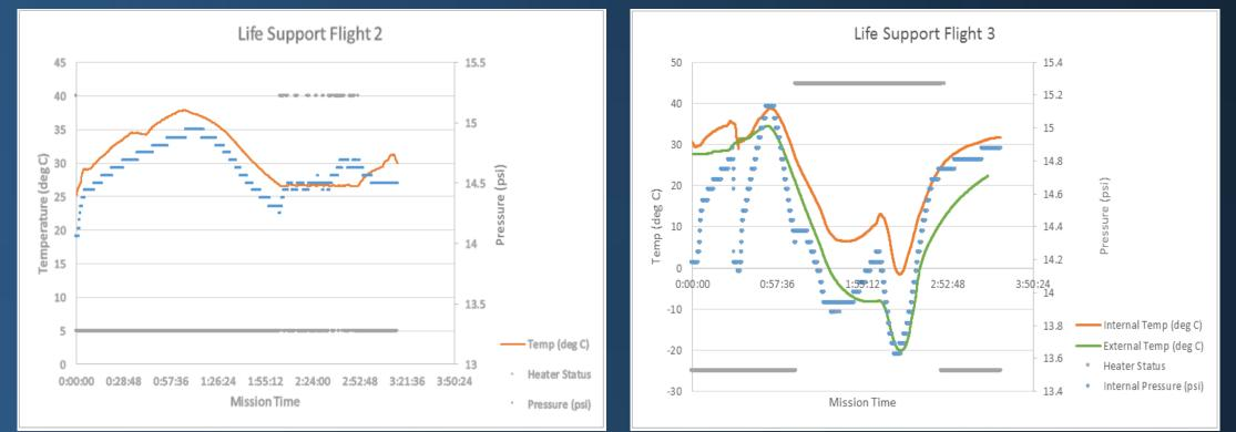
The second flight was much more successful, with the crickets (and sowbugs included on this flight) surviving. However, the camera overheated just before launch, so no video was recorded. On the third flight, flown without insulation, the heater was not quite capable of keeping up with the low external temp. so the internal temp. dropped to just below freezing. Despite this, the crickets still survived. We are considering future flights with this payload.
