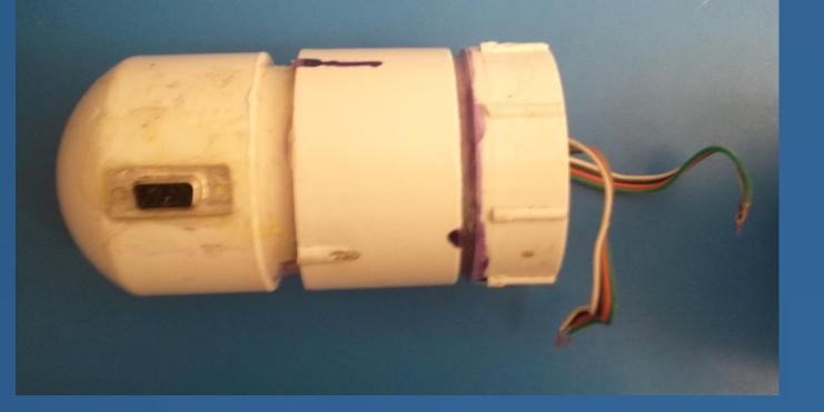
The second version, which was built and is pictured above, is essentially a scaled-down version of the first concept. The Arduino and camera were moved out of the chamber, and the crickets would be viewed through a Plexiglas window. The internal heater and sensors would be connected with electrical feed-throughs in the chamber wall.
