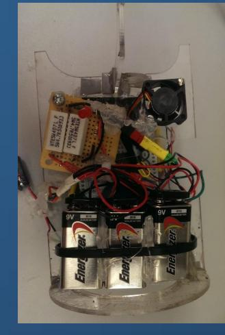
For the first flight, the electronics, batteries, and cricket holder were simply hot-glued in place. However, turbulence just after burst led to the glue attachments failing. In later flights a removable 'sled' for mounting electronics was built from laser-cut acrylic sheets (see above).
