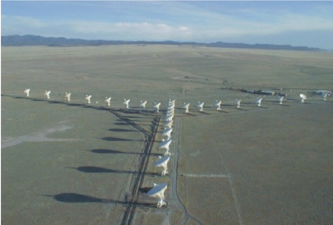
Figure 1.4: Photograph of the EVLA, located in New Mexico (courtesy of the NRAO – a facility of the NSF operated under cooperative agreement by Associated Universities Inc.). Each individual EVLA antenna has a diameter of 25 m, which is much smaller than the diameter of the Arecibo single dish (305 m). Using the technique of interferometry (described in Section 1.2), signals received by the EVLA antennas can be combined so that the array performs like a single telescope with an equivalent dish diameter equal to the maximum distance between the antennas. The telescopes are mounted on railroad tracks to allow the spacing to be modified into four different configurations or arrays. In the picture the EVLA is in D configuration where the antennas are as close together as possible. Being able to change the distance between antennas allows the resolution to be adjusted, and in A configuration (when the antennas are separated by the most distance) the EVLA has a much better resolution than Arecibo ( 0.24'' in X-Band to 1.4'' in L-Band, see Section 2.1 for more information on the EVLA).
