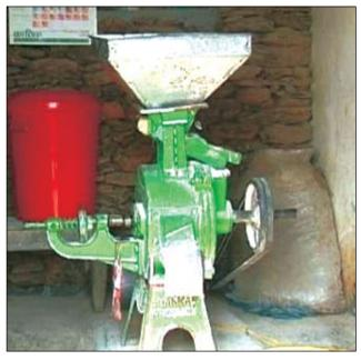
Fig. 8. Community operated micro-mill used in villages
