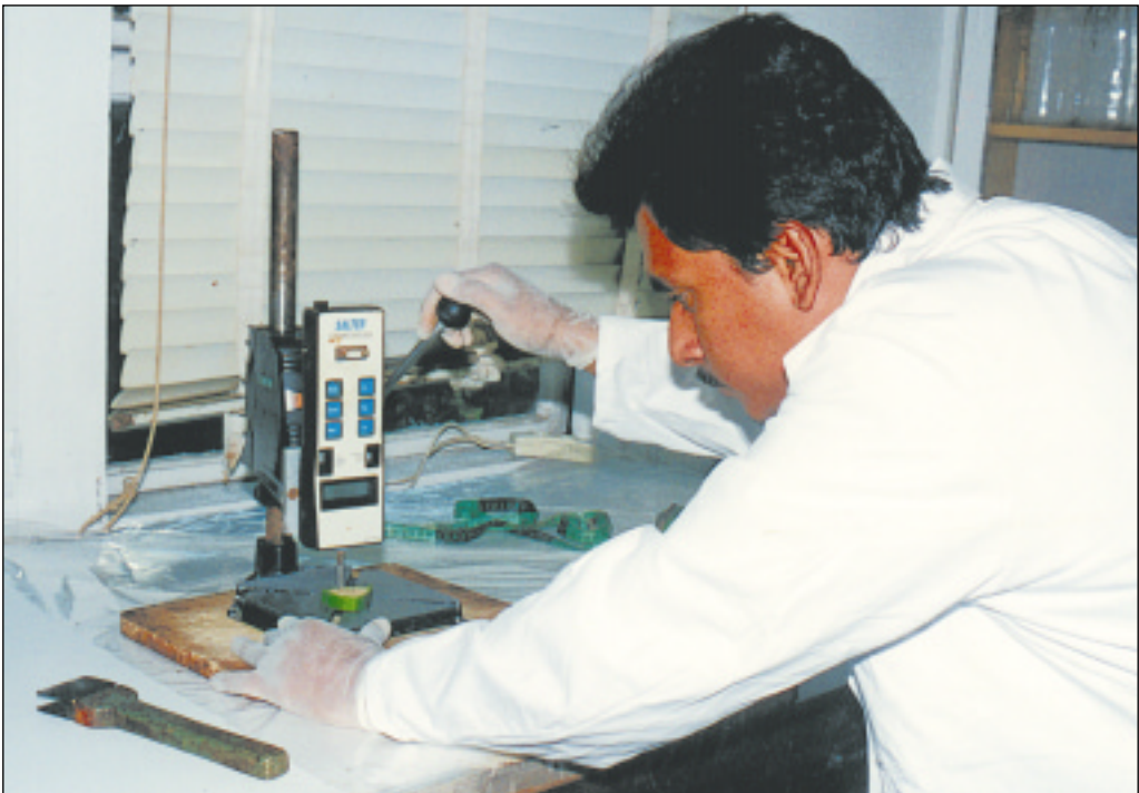
Figure 5: Using bench-top firmness tester fitted with a 6 mm probe to measure pulp firmness.
