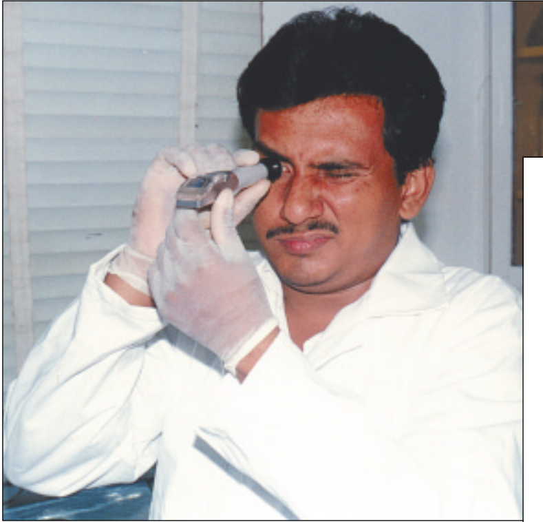
Figure 6: Measuring total soluble solids content with a hand-held refractometer.
