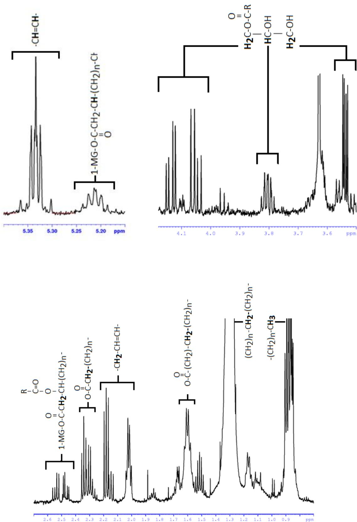
**Figure (6+1)S.** Three enlarged views of the  $^1\text{H}$  NMR of 4b. Relevant signals for the 1-MG are assigned.
