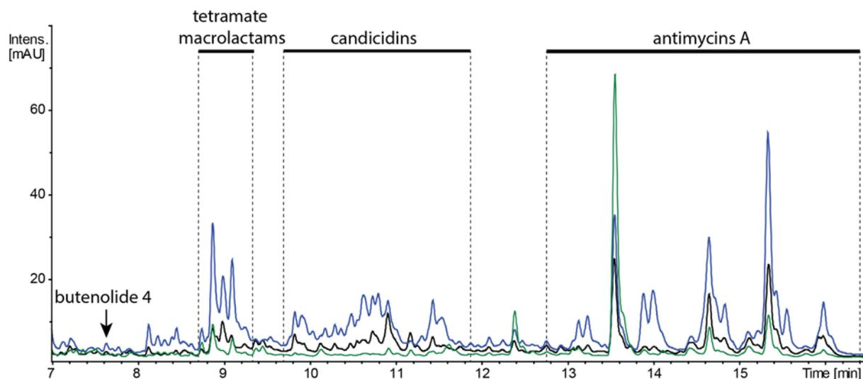
**Figure 4.** LC-MS chromatogram (at 320 nm) of extracts of *S. albus* J1074 (black), *S. albus*  $\Delta$ 3174 (blue) and *S. albus*  $\Delta$ 3174 $\Delta$ 2339 (green). Groups of identified compounds are highlighted. Metabolites were separated with a 20 min gradient.
