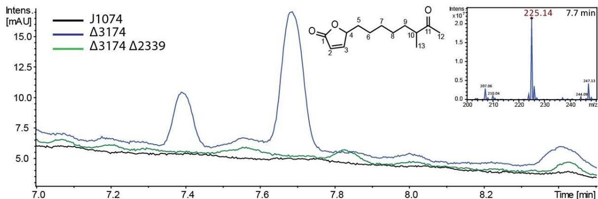
**Figure 8S.** Production of butenolide 4 by strains *S. albus* J1074 (black trace), *S. albus*  $\Delta 3174$  (blue) and *S. albus*  $\Delta 3174 \Delta 2339$  (green). Chromatogram of 20 min gradient protocol (see Materials and Methods) at 320 nm is shown. Compound with retention time of 7.7 min was purified and its structure was proved with the NMR.
