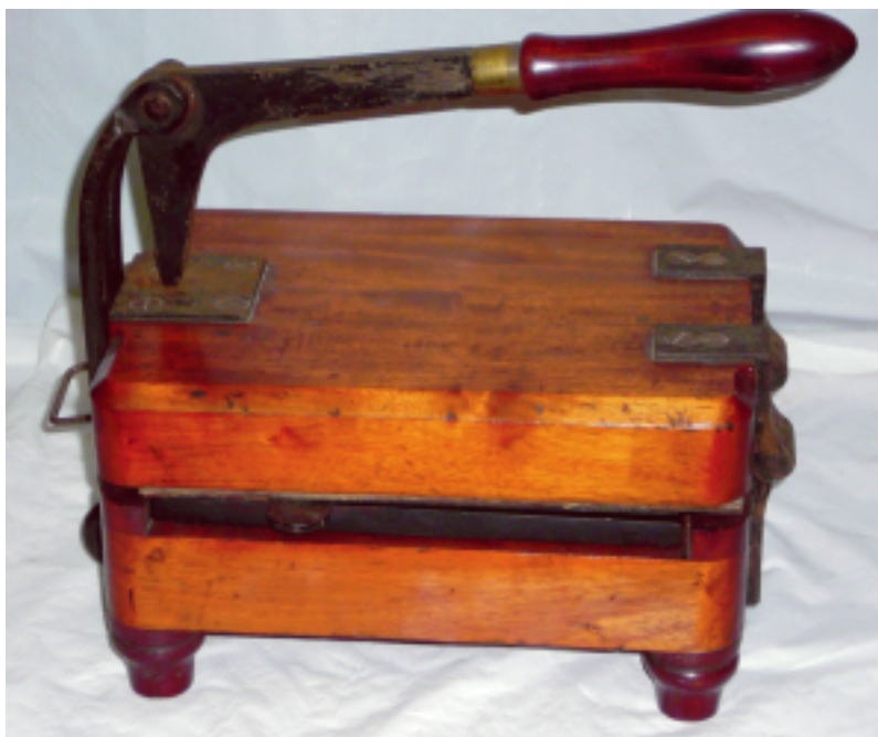
Fig. 3. Example of a standard model Cowper parlour press at the Platen Press Museum, Zion, Illinois, side view, closed (photograph by Paul Aken).
