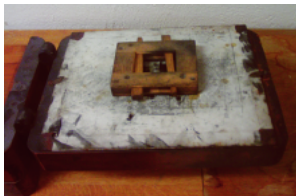
Fig. 7. Platen and tympan of the Cowper parlour press at the Oxford University Museum of Natural History, with an improvised miniature wooden chase attached.
