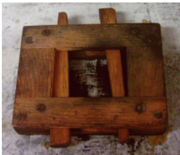
Fig. 8. The improvised miniature wooden chase attached to the Cowper parlour press at the Museum of Natural History, Oxford.
