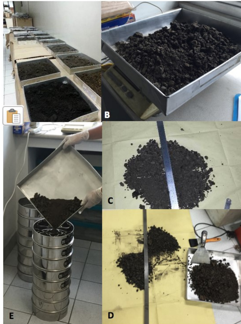
Figure 3.8. Grain size processing of the AD1754 tephra deposits included: (A) air drying of samples; (B) weighing of samples before and after drying; (C) and (D) mixing and splitting of samples using coning and quartering with two of the quarters used for grain size analysis using the Tyler Standard sieves from -6\phi to +4.5\phi at 1/2\phi interval; and (E) manually sieving because the scoria fragments are too fragile and could easily be crashed if mechanical sieving were used.
