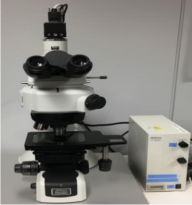
Figure: 2.7 Set up of Interference Microscopy (Nikon- Eclipse LV150N) utilized for thickness measurement.
