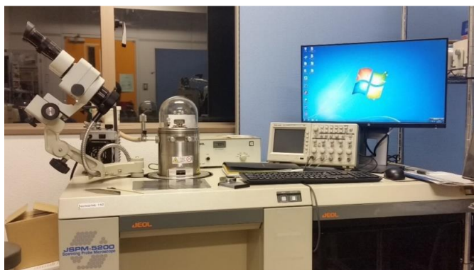
Figure: 2.10 Set up of AFM system with JEOL-SPM used for AFM measurement.
