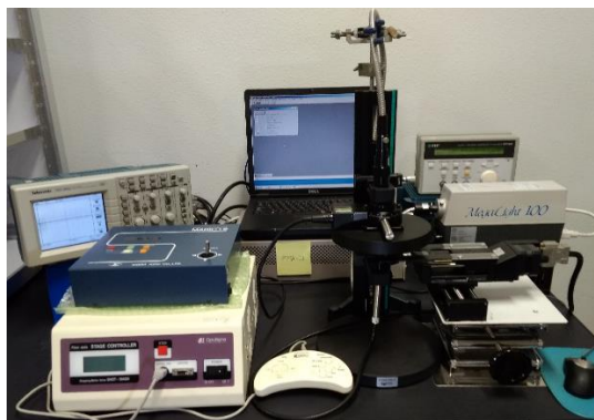
Figure: 2.8 2 D position mapping set up used for analysis of thin film distribution.
