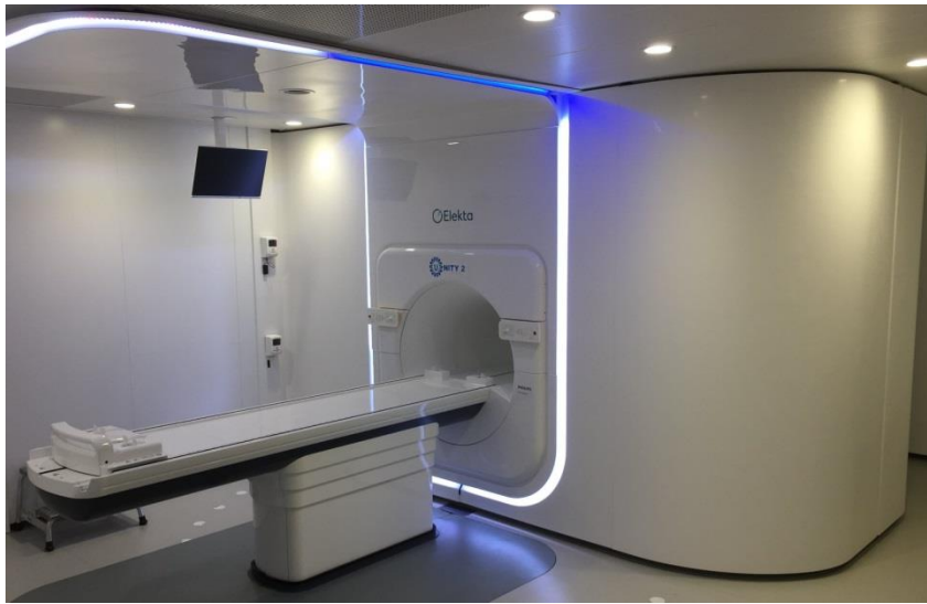
Figure 2: (a) Elekta's 1.5 Tesla Unity system at University Medical Centre in Utrecht, The Netherlands; This was the MRI-Linac used for the first in man treatments in May 2017 (courtesy of Bas Raaymakers, UMC).
