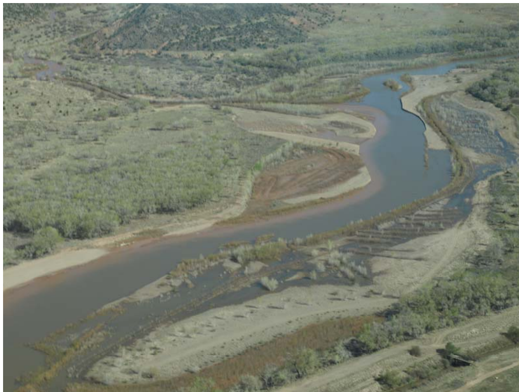
Photo 9: Looking upstream at location of sediment spoil pile on the Pueblo of Santa Ana after sediment has been removed. Flow in the Rio Grande is approximately 3000 cfs (April 2010, Holste)
