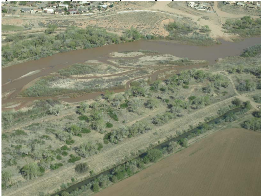
Photo 12: Looking west at Corrales Siphon river maintenance site location during spring runoff. Note high flow channels cut in bar by Pueblo of Sandia. Flow in the Rio Grande is approximately 3000 cfs. (April 2010, Holste)
