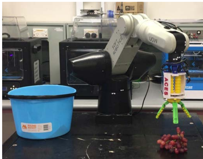
Fig. 7. CRS 6-DOF robotic manipulator with OPSOG
