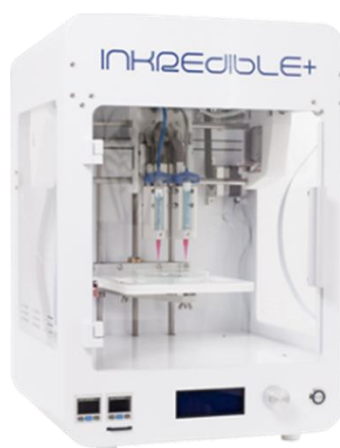
Fig 5-2: Image of the INKREDIBLE+ Bioprinter utilised for all bioprinting experimental work outlined in this chapter.
