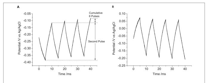
**FIGURE 3** | Multiple pulse chronopotentiometry of a mechanically polished 0.6 mm diameter platinum electrode in degassed 0.1 M NaCl. **(A)** Cathodic, **(B)** anodic pulse first with a current density of 10  $\mu$ C cm<sup>-2</sup>.
