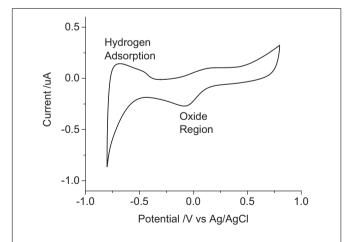
**FIGURE 1** | Second cycle of a cyclic voltammogram in degassed 0.1 M NaCl of a mechanically polished 0.6 mm diameter platinum electrode at 100 mV s $^{-1}$ .
