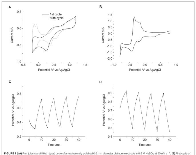
an acid polished 0.6 mm diameter platinum electrode in degassed 0.1 M NaCl at 100 mV s<sup>-1</sup>. Multiple pulse chronopotentiometry of an acid polished 0.6 mm diameter platinum electrode in degassed 0.1 M NaCl. **(C)** Cathodic, **(D)** anodic pulse first with a current density of 10  $\mu$ C cm<sup>-2</sup>.
