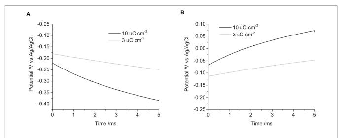
**FIGURE 2** | Chronopotentiometric curves of a mechanically polished 0.6 mm diameter platinum electrode in degassed 0.1 M NaCl. (A) cathodic pulse, (B) anodic pulse. Black curve – current density of 10  $\mu$ C cm<sup>-2</sup>, Gray curve – 3  $\mu$ C cm<sup>-2</sup>.
