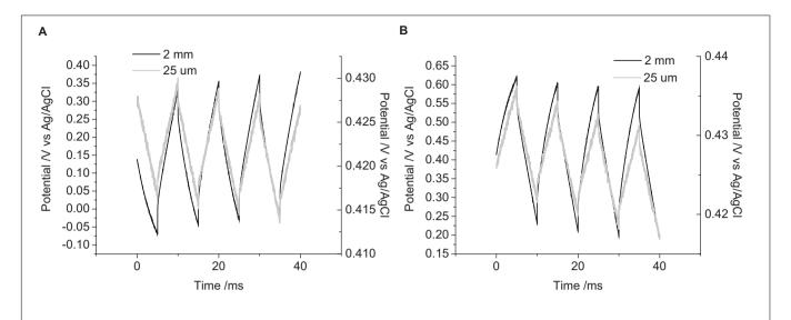
FIGURE 6 | Multiple pulse chronopotentiometry of a mechanically polished platinum electrode in 0.1 M NaCl in degassed 0.1 M NaCl. (A) Cathodic, (B) anodic pulse first with a current density of 10 μC cm<sup>-2</sup>. Black curve – 2 mm diameter electrode, Gray curve – 25 μm diameter electrode.
