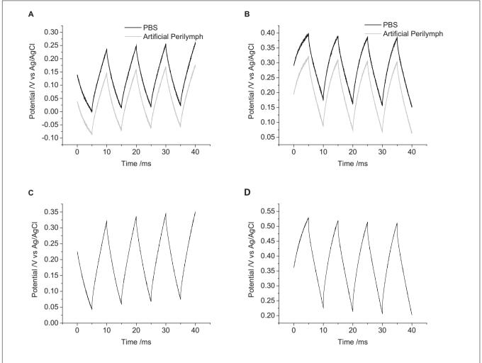
**FIGURE 5** | Multiple pulse chronopotentiometry of a mechanically polished 0.6 mm diameter platinum electrode. **(A)** Cathodic, **(B)** anodic pulse first with a current density of 10  $\mu$ C cm<sup>-2</sup> in degassed solution. Black curve – PBS, Gray curve – artificial perilymph. **(C)** Cathodic, **(D)** anodic pulse first with a current density of 10  $\mu$ C cm<sup>-2</sup> in non-degassed 0.1 M NaCl.
