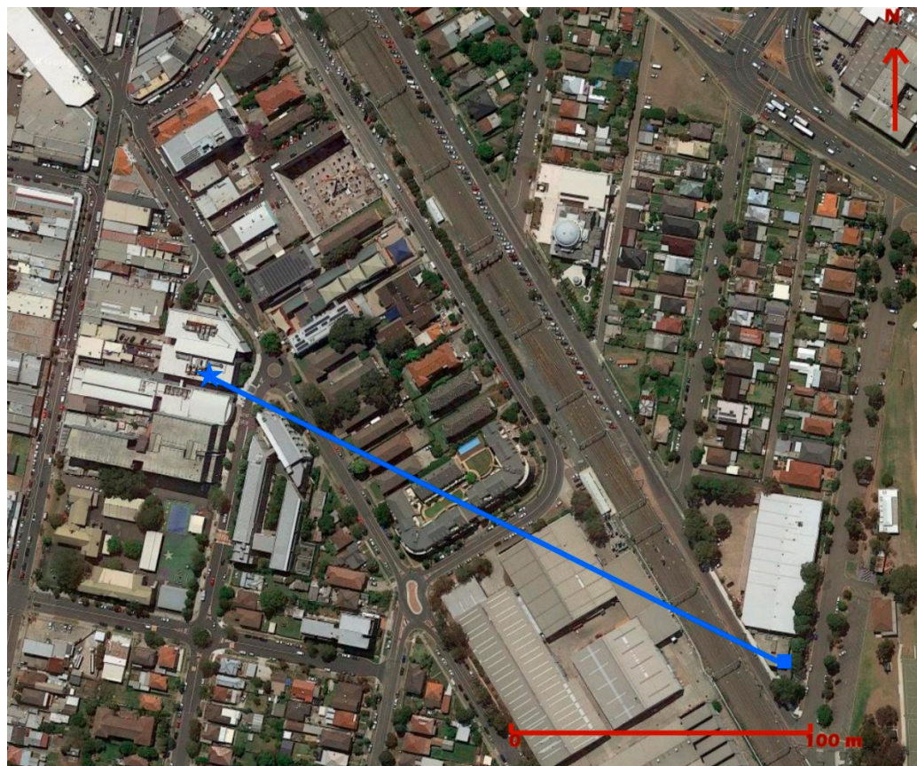
Figure 1. The measurement site at the edge of the Auburn business district. The location of the main measurement site including the open path Fourier transform infra-red (OP-FTIR) spectrometer location (□), on roof of 2 story building and retro-reflectors (★) on roof of 3 story building at the edge of the small business district in Auburn is located. The measurement path (395 m) is marked (-). There is a major intersection in the north-east. To the east is light industrial area, with mainly residential to the east. The measurement path crosses a railway line and a major intra-urban motorway is to the east (not shown on the map).
