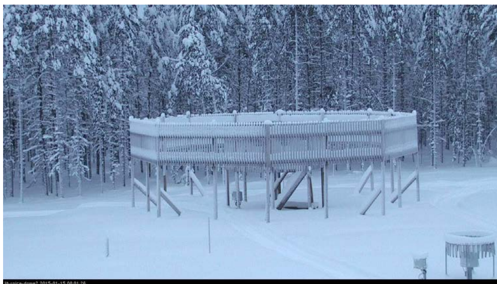
Figure 4.116. Snow accretion on instruments and various structures (DFIR, SA shield) at Sodankylä.
