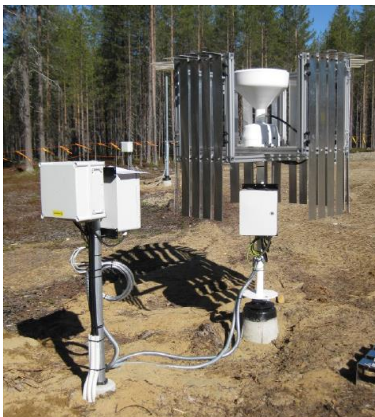
Figure 4.29. EML UPG1000 heated tipping bucket gauge under test at Sodankylä with wind shield.
