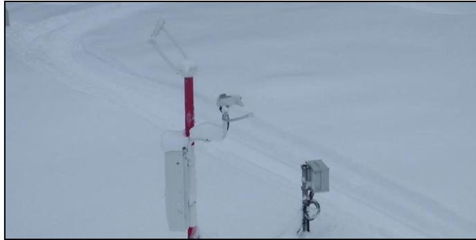
Figure 14: Snow accumulation on FS11P device, 2015-02-15, 11:03 UTC.
