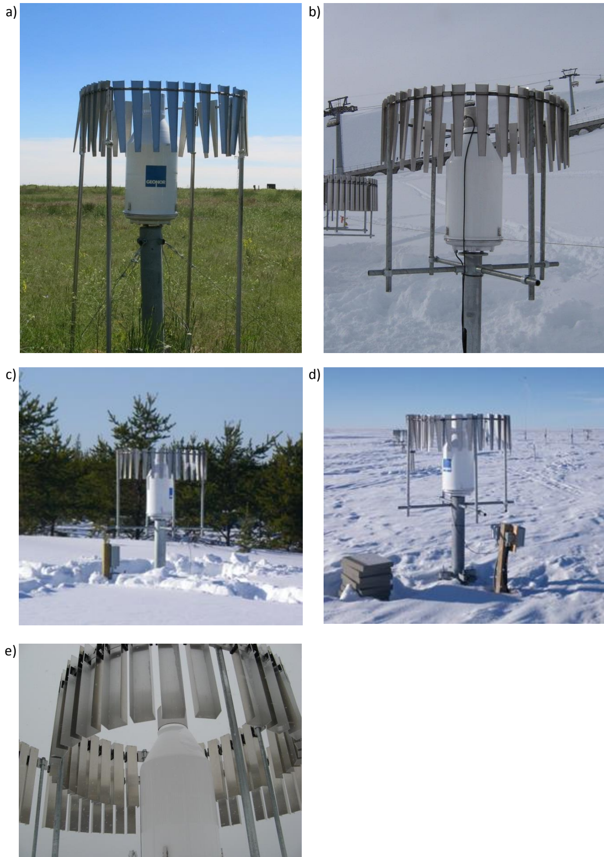
Figure 1: Geonor T-200B3MD test gauges in single-Alter shields at (a) Marshall (USA), (b) Weissfluhjoch (Switzerland), (c) Caribou Creek (Canada), and (d) Bratt's Lake (Canada), and (e) in Belfort double-Alter shield at CARE (Canada).
