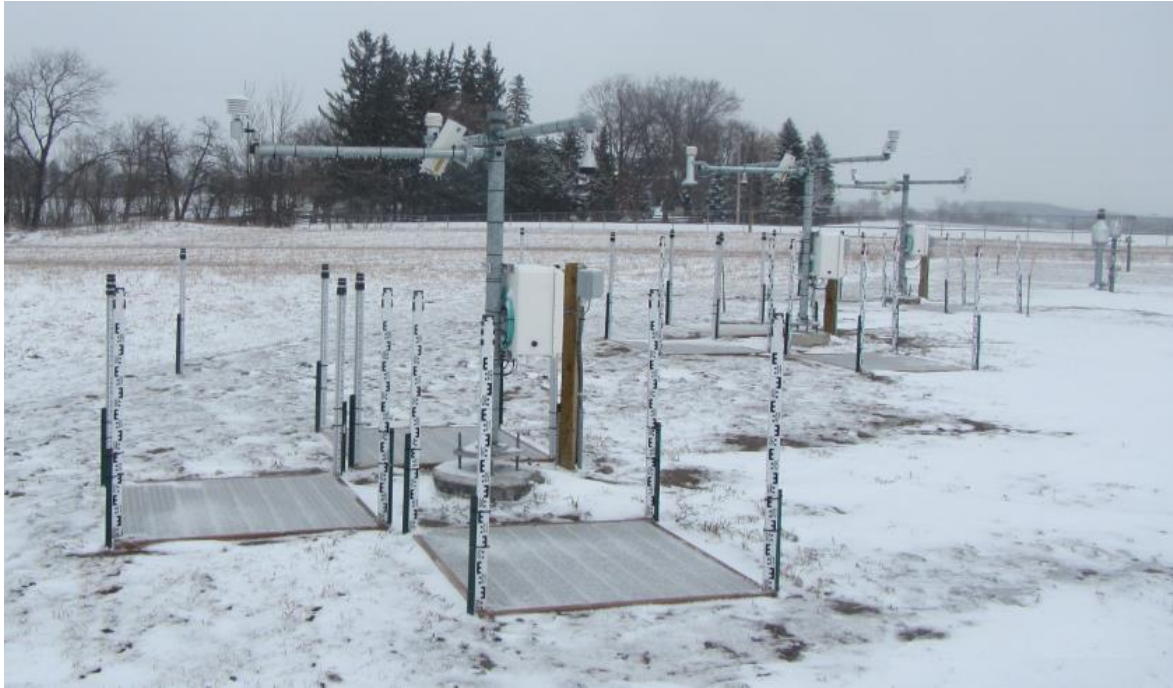
Figure 3.15. Configuration of the STR0a reference configuration at CARE, with snow stakes at the four corners of the surface target, just outside the FOV of each automated sensor.
