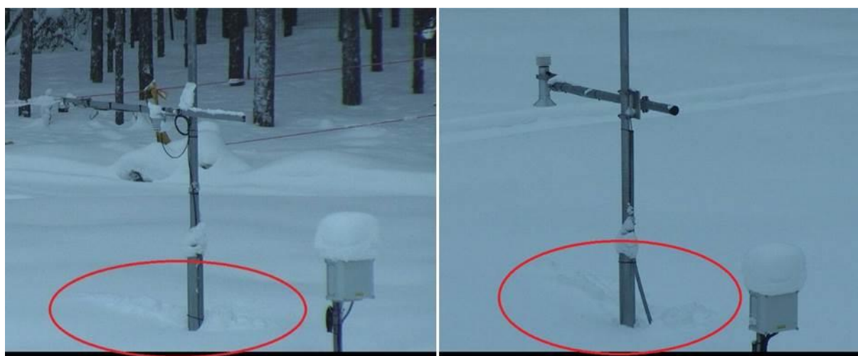
Figure 4.171. The impact of snow falling off horizontal unheated instrument booms at Sodankylä following a heavy snowfall event. The fallen snow in the target area is circled in red.
