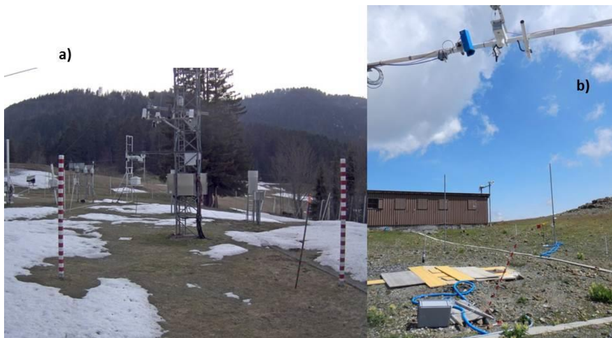
Figure 4.179. Natural ground targets under the snow-depth sensors at a) Col de Porte (mown grass), and b) Weissfluhjoch (grass and rock).
