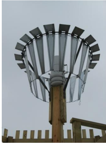
Figure 3.2. Tretyakov gauge and shield (CARE, Canada).
