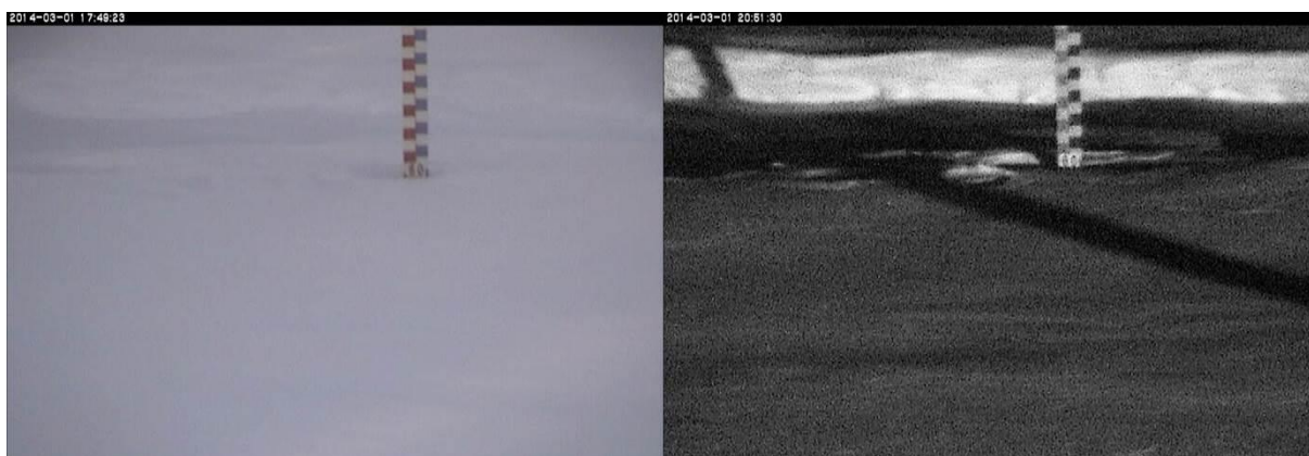
Figure 3.16. Example of hourly photos of the snow stakes at Caribou Creek during the day (left) and night (right).
