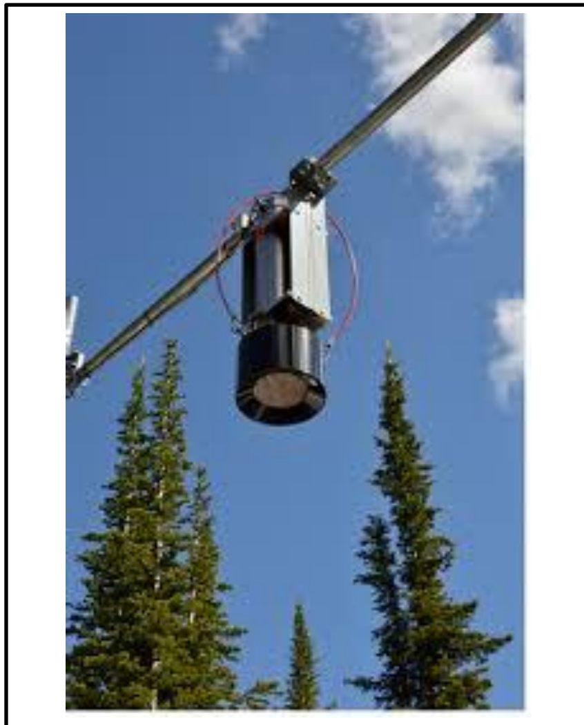
Figure 1: Photo of the CS725 SWE sensor
