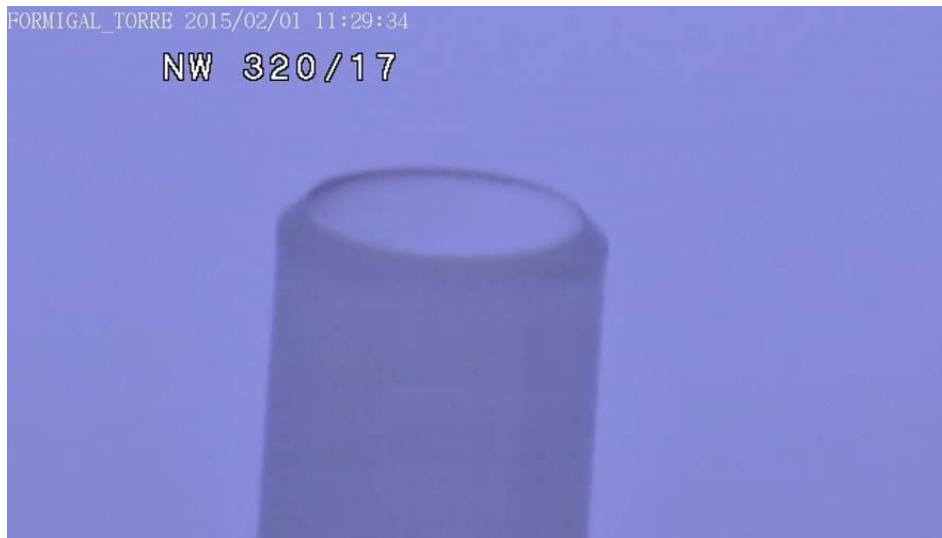
Figure 4.115. Capping observed in Thies tipping bucket, Formigal site on February 1, 2015.
