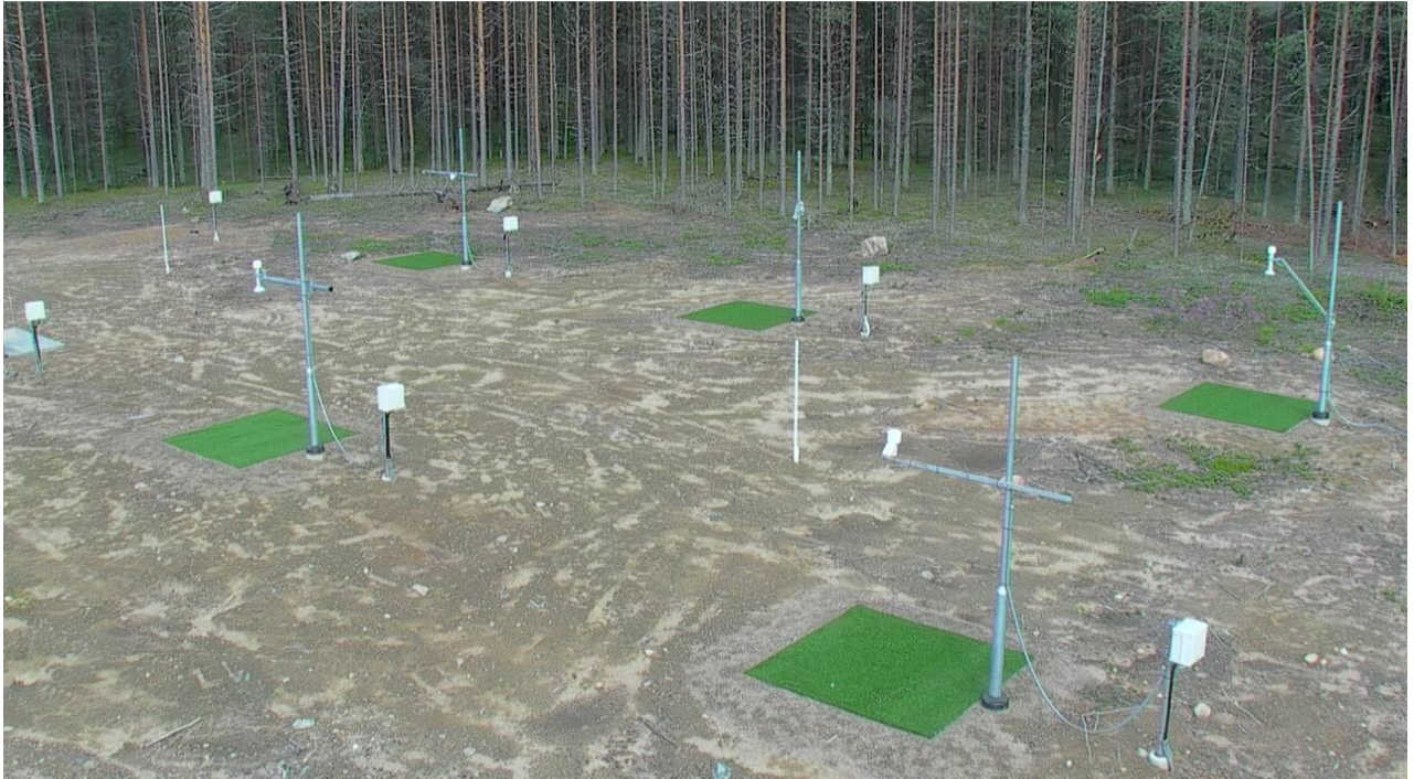
Figure 4.178. Artificial targets in the SPICE intercomparison field at Sodankylä.
