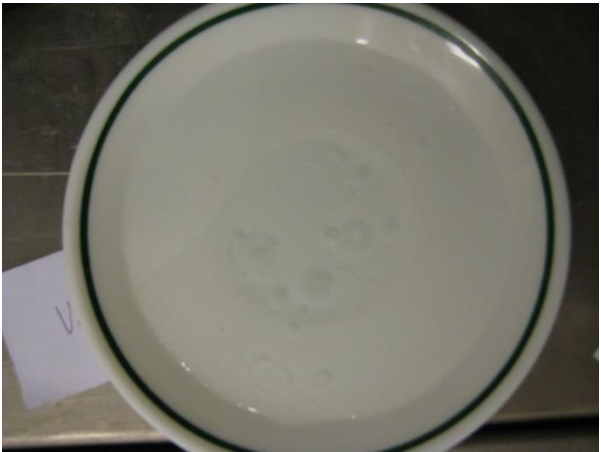
Figure 11: water droplets agglomerate in Vaseline.
