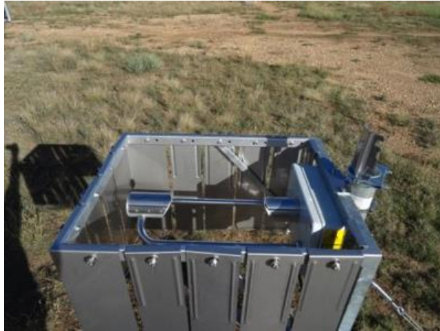
Figure 4.51. Thies LPM sensor at the Marshall site with wind shield.
