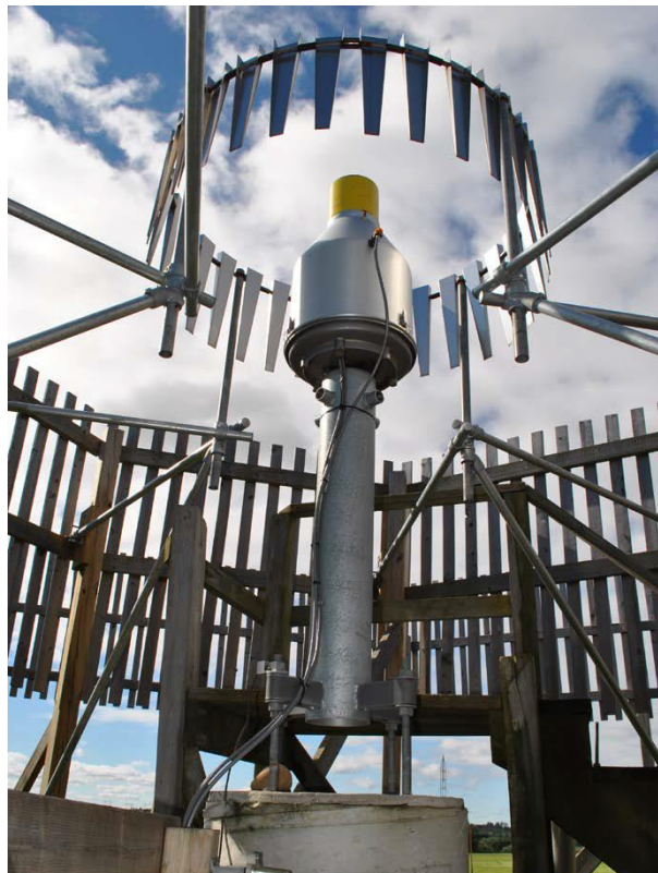
Figure 3.34. Geonor T-200B3 gauge in R2 reference configuration at the CARE site.
