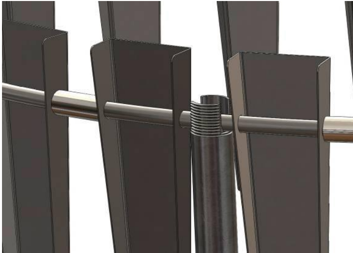
Figure 8: Support post and rod mounting - view 1
