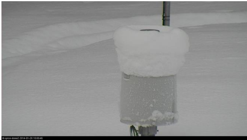
Figure 4.146. Buildup of snow on the shoulders of an OTT Pluvio 2 gauge at Sodankylä employing rim heating and the OTT heating algorithm.
