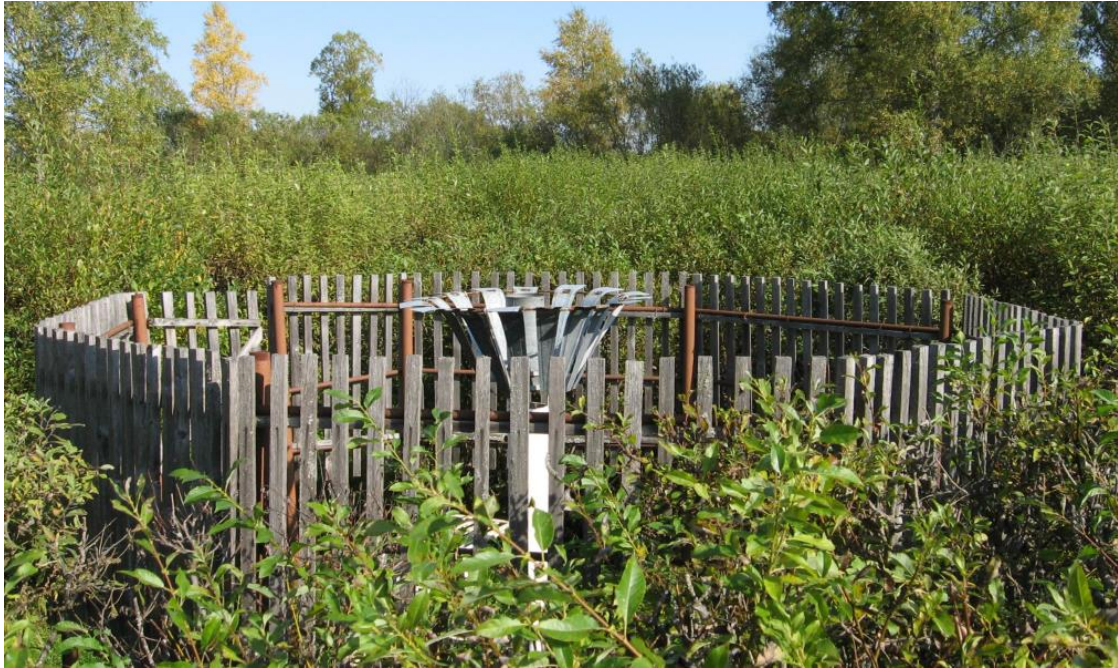
Figure 3.5. Field working reference system type R0 (the bush gauge) as configured at the Valdai SPICE site, Russian Federation.
