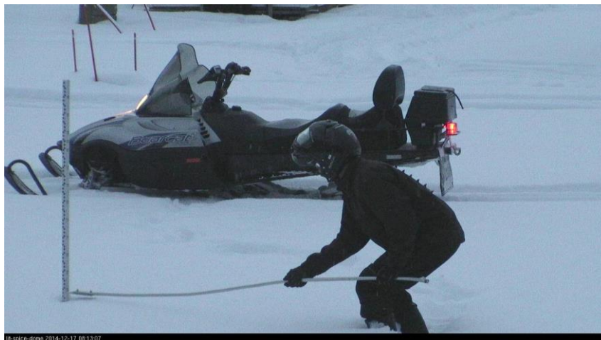
Figure 3.17. Leveling a mound around a snow stake at Sodankylä during site maintenance.
