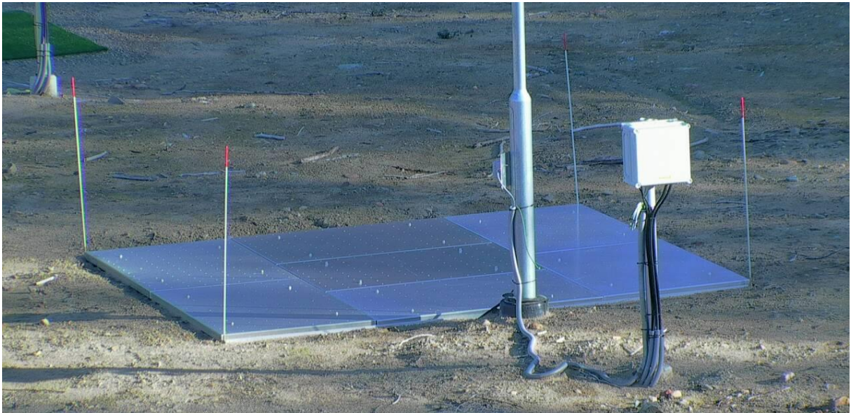
Figure 3: Sommer Messtechnik SSG1000 snow scale at the Sodankylä SPICE intercomparison site.
