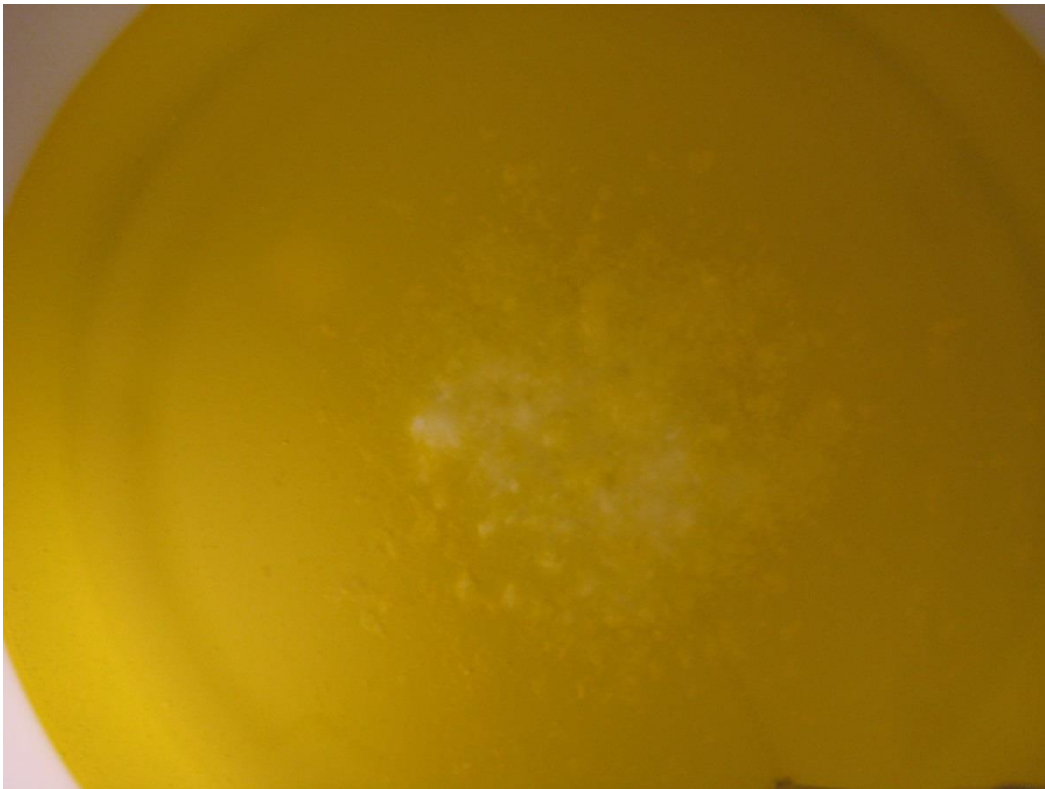
Figure 3: frost and water droplets remain on the surface of the linseed oil.
