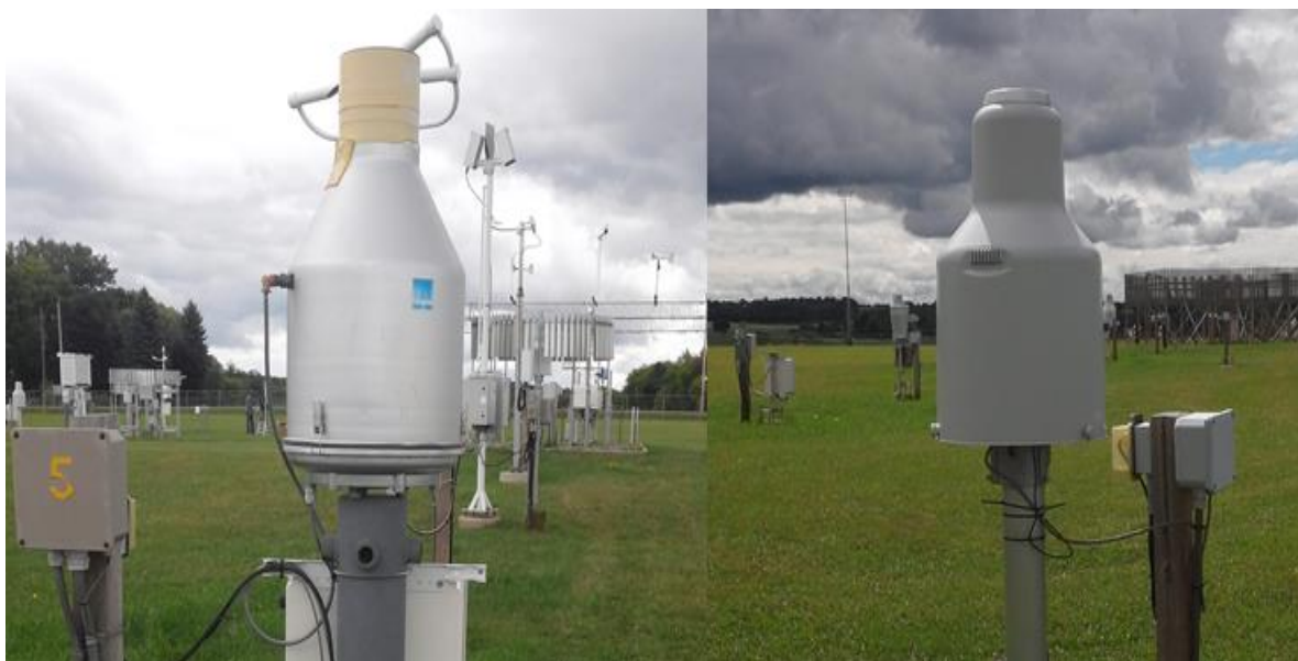
Figure 3.46. Weighing gauges used in R2 reference configurations: (a) Geonor T-200B3, (b) OTT Pluvio 2 (photos from CARE SPICE site).
