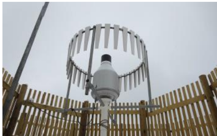
Figure 5 Geonor T200B in the double fence.
