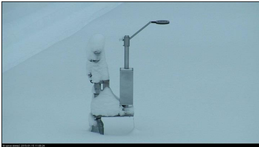
Figure 17: No snow accumulation observed on the Hotplate device at Sodankylä site despite an important snowfall, 2015-02-15, 11:00 UTC.
