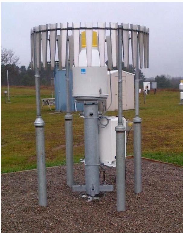
Figure 2: Single Alter Shield Mounting, R3(G,SA) Reference, CARE, Canada
