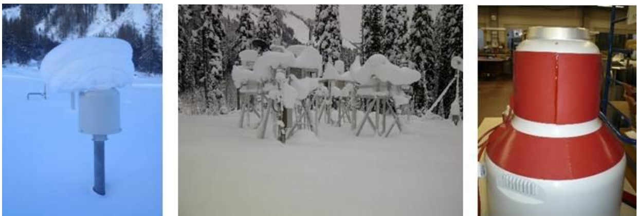
Figure 4.135. a) Capping in a location with limited power resources (Switzerland), b) Huge capping in a forested area in British Columbia (Canada), c) Thermal blanket in laboratory testing (Meteoswiss).
