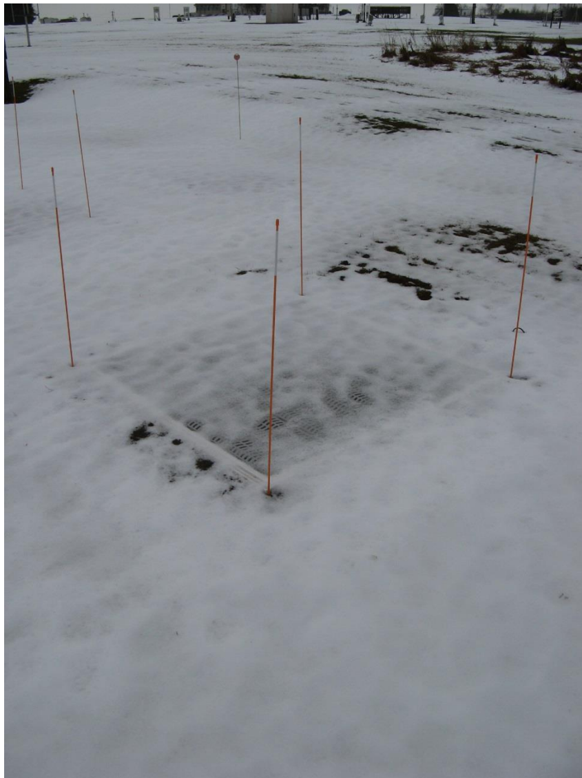
Figure 4.183. Experimental plastic target at CARE taken on December 17, 2014, after a snowfall event on the bare ground and targets. Photos obtained during a pre-SPICE target assessment project (Courtesy of Jeffery Hoover, Environment and Climate Change Canada).
