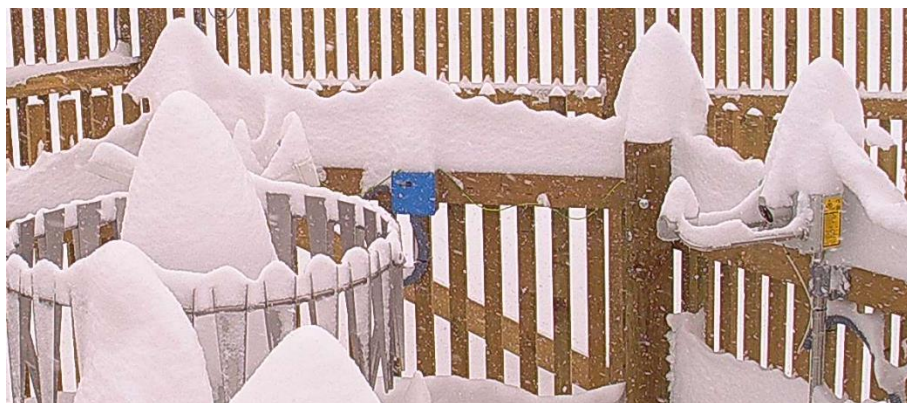
Figure 4.112. Severe capping of Pluvio 2 in DFIR, Formigal, February 2, 2015.
