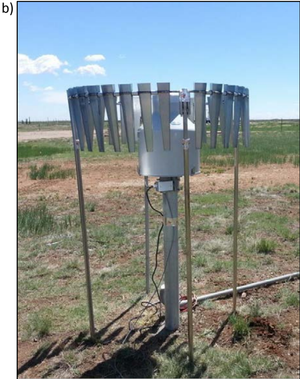
Figure 1: Sutron TBG gauges under test in (a) unshielded and (b) single-Alter shielded configurations at Marshall site.
