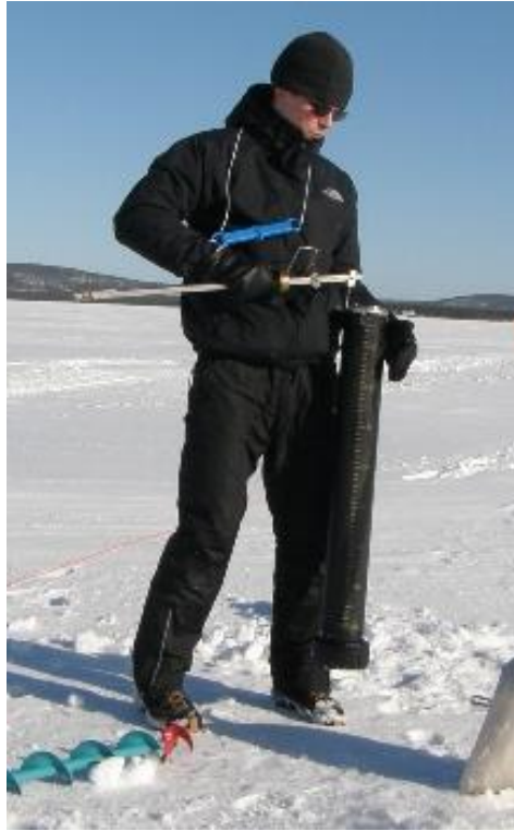
Figure 3.19. Bulk-density SWE measurement using a Finnish Korhonen-Melander snow sampler.
