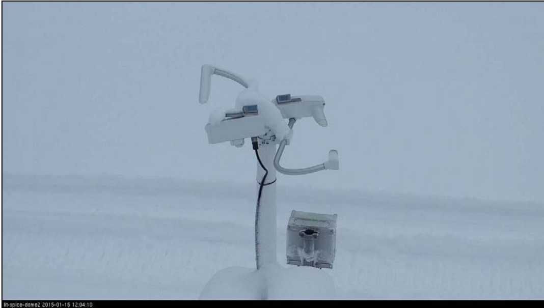
Figure 15: Snow accumulation on PWD33 EPI device, 2015- 02-15, 11:02 UTC.
