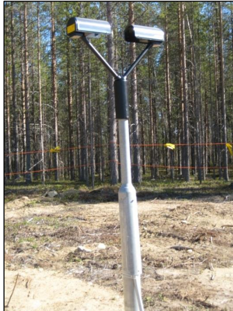
Figure 1: Parsivel 2 at Sodankylä test site.
