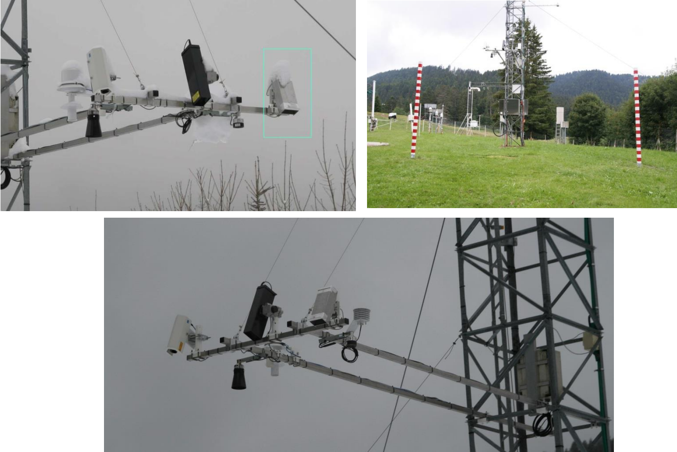
Figure 3: Dimetix FLS-CH 10 on the SPICE beam at Col de Porte
