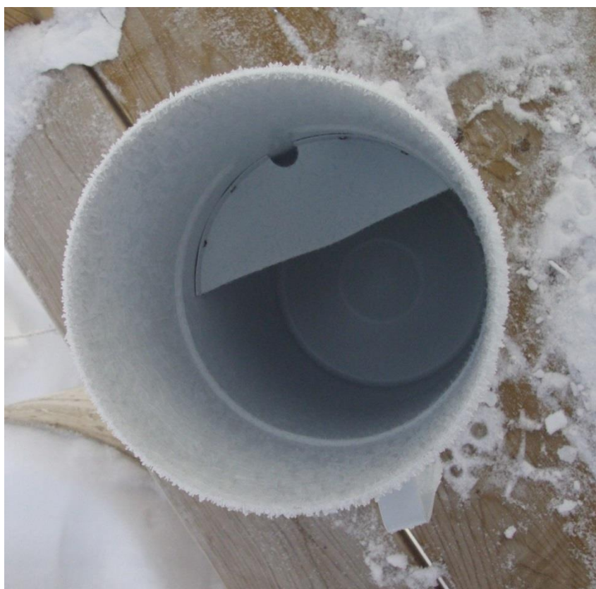
Figure 3.40. Frost on the R1 manual gauge at CARE. (Photo credit: P. Raczynski)
