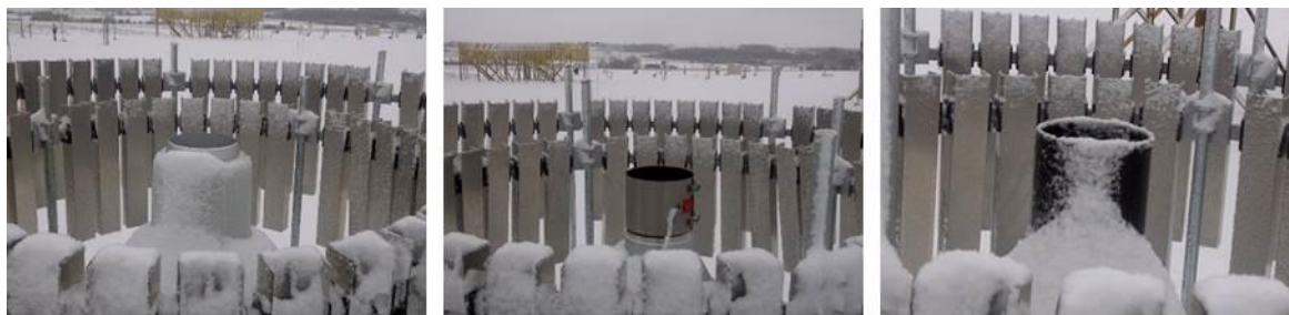
Figure 4.122. Accretion of snow on heated Pluvio 2 (left), heated Geonor (center) and unheated Geonor (right) at CARE in December, 2014. All gauges are in double-Alter shield configurations.
