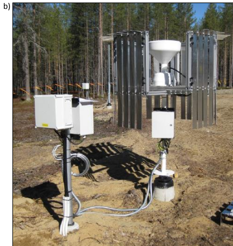
Figure 1: EML UPG1000 installation at (a) Marshall, with vertical shield slats, and (b) Sodankylä, with L-shaped shield slats.
