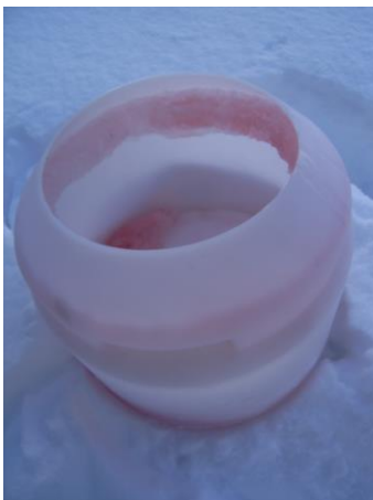
Figure 1 : Picture of the Pluvio 2 bucket after the emptying of the bucket, showing an ice ring (containing some oil hence the red color) on 31 January 2014.
