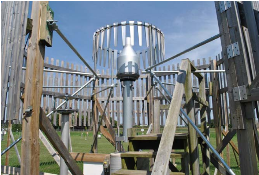
Figure 1: Single Alter Shield Mounting in DFIR, R2(G,SA) Reference, CARE, Canada
