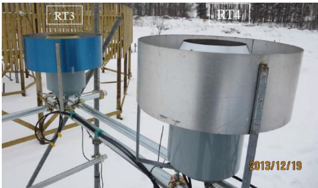
Figure 9 Tipping buckets, RT3 and RT4. The mechanism of measurement in each instrument is illustrated in Figure 10.
