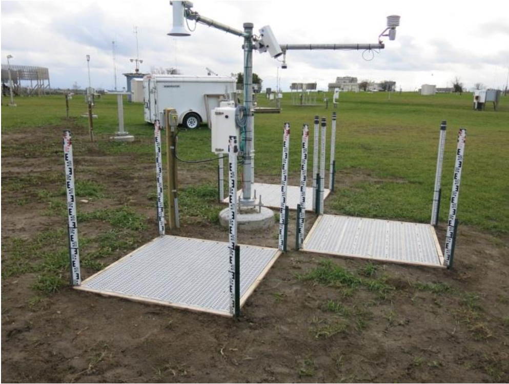
Figure 4.175. Completed target installation at one of the three snow depth measurement pedestals at CARE.
