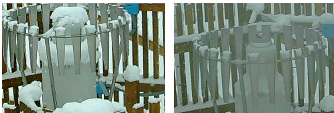
Figure 4.125. Pluvio 2 in the DFAR at Formigal with rim heating off (left) and after turning on the rim heating (right) on November 25, 2015.
