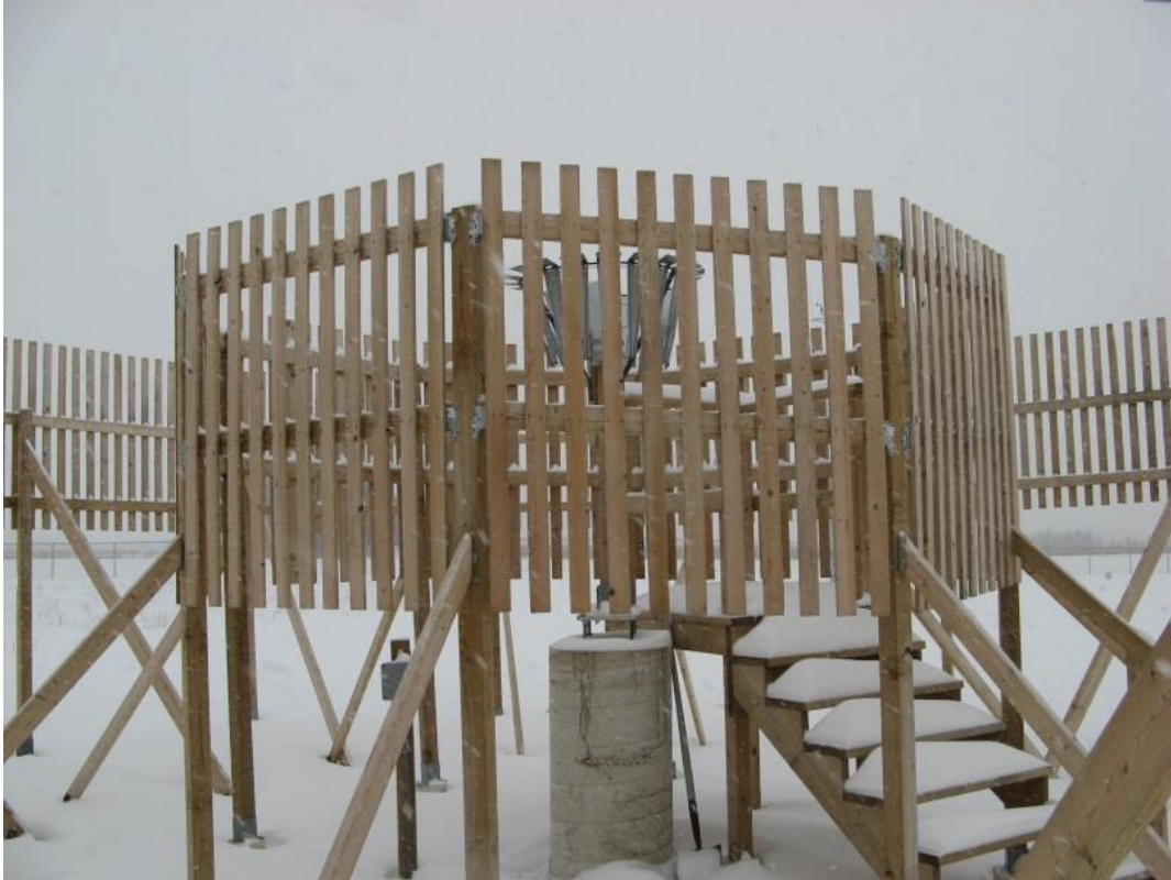
Figure 3.7. Field working reference system type R1, as configured on the CARE SPICE site, Canada.
