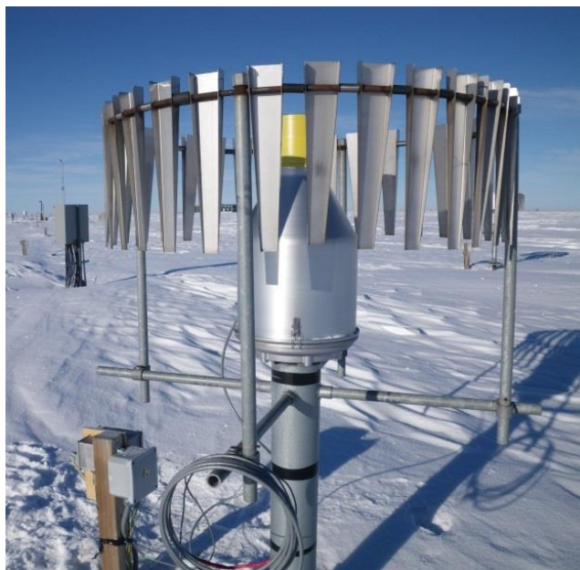
Figure 3.12. Single-Alter shield (Bratt's Lake SPICE site, Canada).
