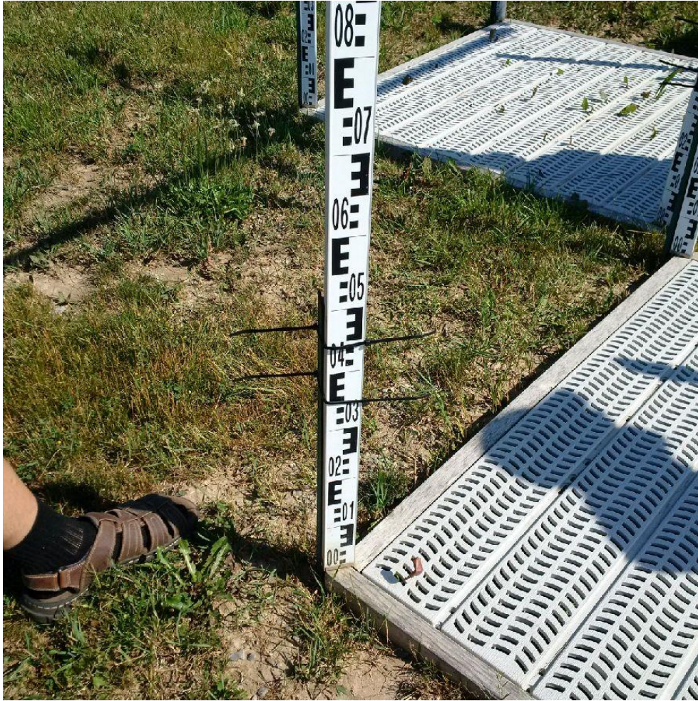
Figure 3.21. Photo of the artificial snow-depth target at CARE and the manually observed snow stake on one corner. The snow targets were originally installed flush with the ground, but frost heave eventually pushes the target out of the ground and closer to the sensor.
