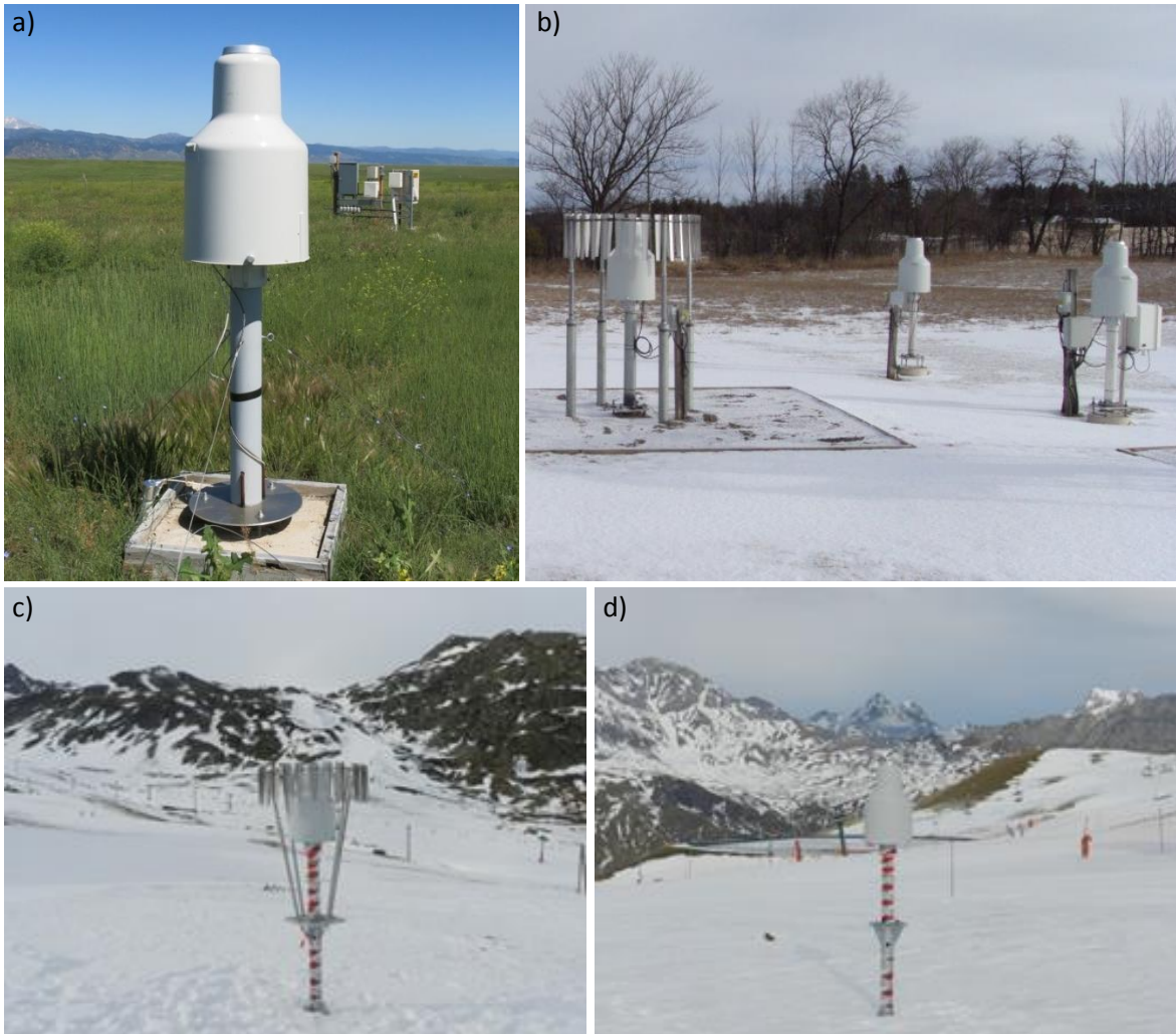
Figure 1: OTT Pluvio 2 test gauges at (a) Marshall (unshielded), (b) CARE (unshielded and single-Alter shielded), (c) Formigal (single-Alter shielded) and (d) Formigal (unshielded).
