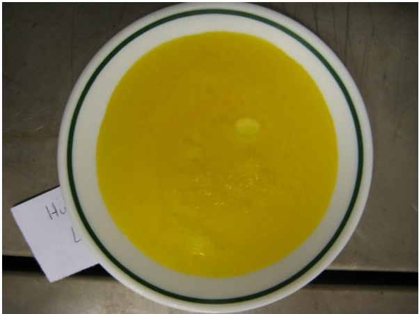
Figure 10: water and frost captured in linseed oil.
