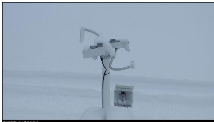
Figure 14 : Snow accumulation on PWD52 device, 2015-02-15, 11:02 UTC.
