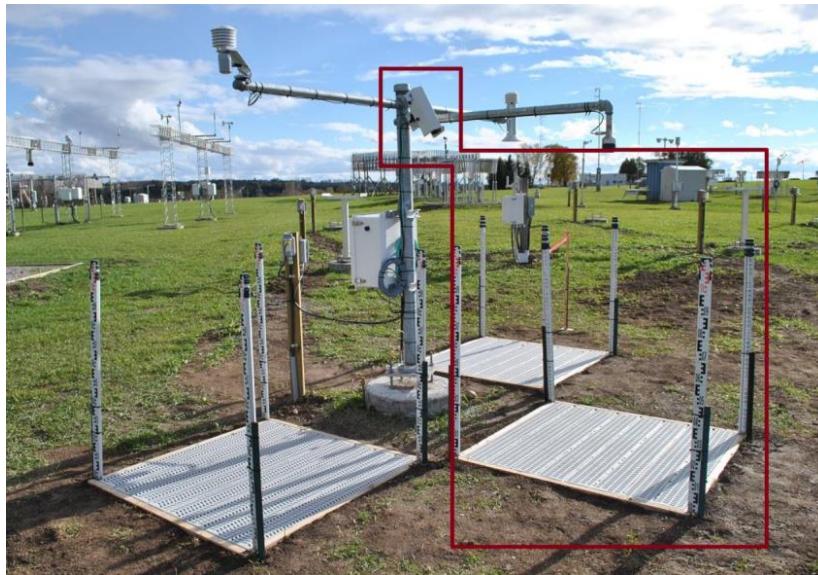
Figure 4.95. Photo of the snow-free target under the snow-depth sensors at CARE. The area outlined in red shows an SHM30 sensor and its target.
