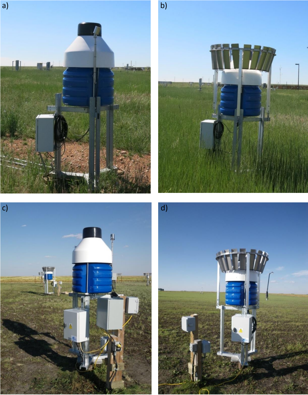
Figure 1: (a) Unshielded and (b) single-Alter/Tret-shielded MRW500 gauges under test at Marshall; (c) unshielded and (d) single-Alter/Tret-shielded MRW500 gauges under test at Bratt's Lake.
