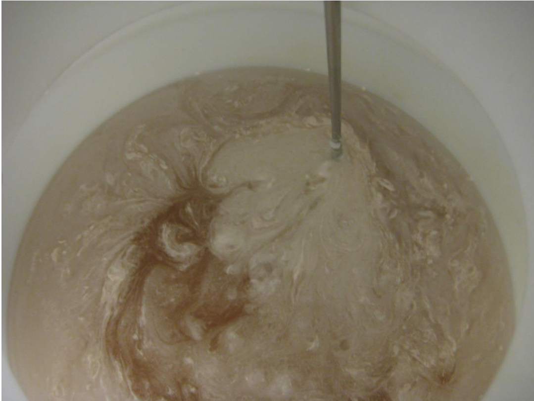
Figure 8: Vaseline layer is easily displaced.
