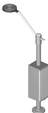
Figure 4.55. Drawing of the TPS 3100 Hotplate sensor, as tested in WMO-SPICE, from the Hotplate User Manual.
