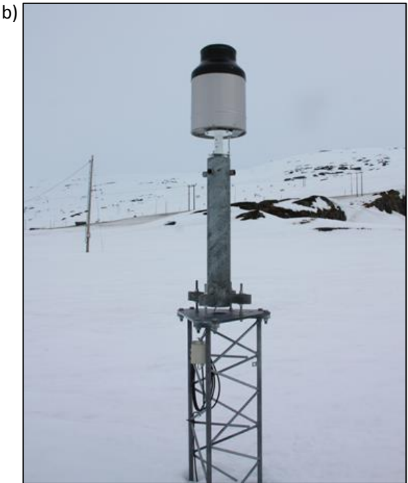
Figure 1: MPS TRwS405 gauges under test at (a) Marshall (USA) and (b) Haukeliseter (Norway).
