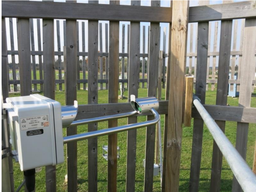
Figure 3.14. This LPM inside a DFIR-fence in R2 FWRS (CARE, Canada).
