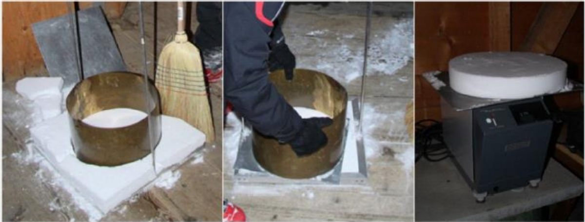
Figure 3.20. SWE measurement at the Weissfluhjoch site using a snow board, sampling cylinder, and scale.
