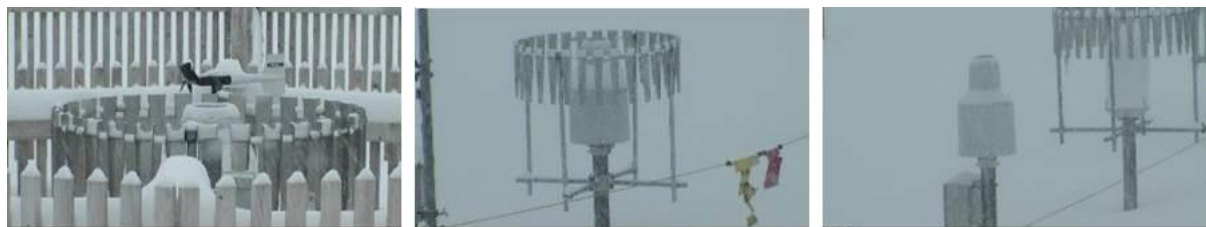
Figure 4.111. Snow accumulation on heated Pluvio 2 in a DFAR (left), in a single-Alter shield (middle) and in an unshielded configuration (right) during a snowfall episode on March 2, 2014 at Weissfluhjoch.
