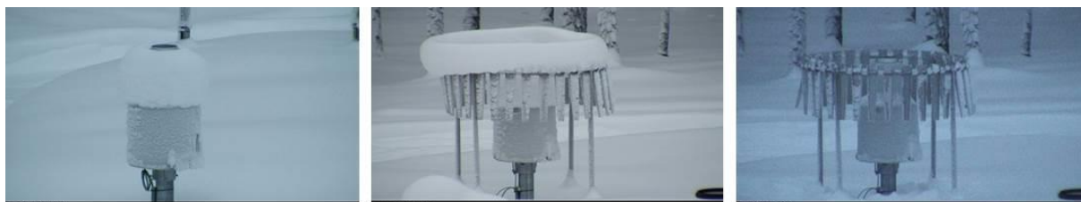
Figure 4.117. Snow capping on unshielded Pluvio 2 (left) and on single-Alter-shielded Pluvio 2 before (middle) and after (right) manual snow removal on January 15, 2015 at Sodankylä.
