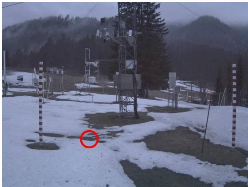
Figure 4.104. Target area under the SHM30 (inside red circle) at Col de Porte, 1845 UTC on April 19, shortly before signal output drops to indicate a snow free target.
