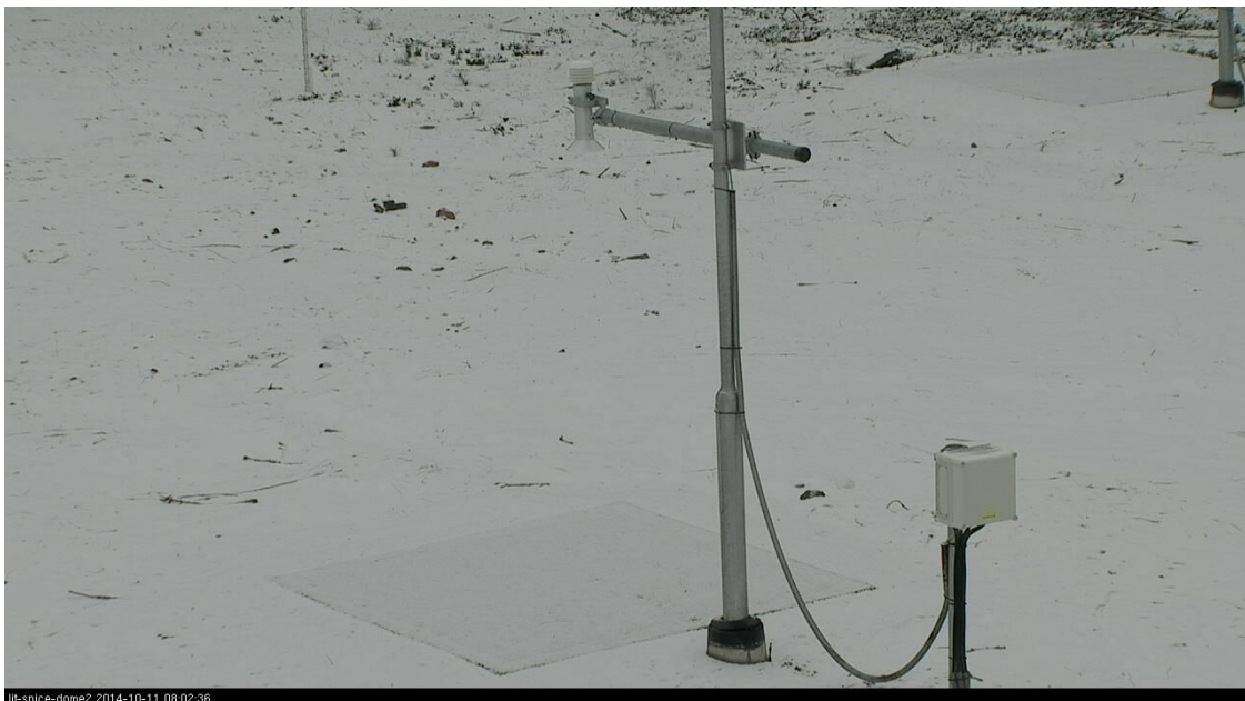
Figure 4.185. Artificial turf targets at Sodankylä during or shortly after a snowfall event on the bare targets October 11, 2014 (observed depths for this event are shown in Figure 4.180b and Figure 4.181b).
