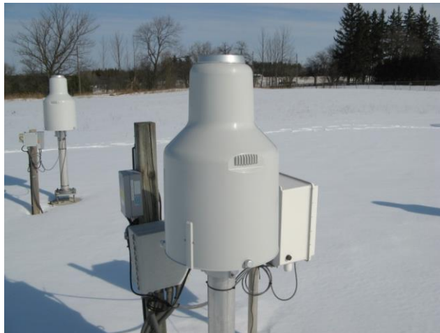
Figure 4.144. OTT Pluvio 2 precipitation gauge with standard heating configuration.
