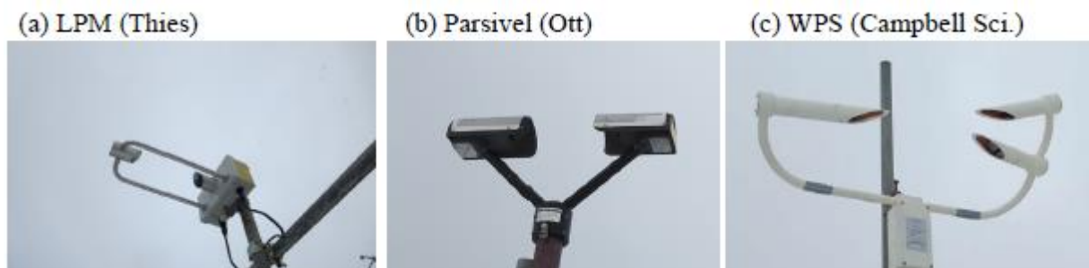
Figure 7 Three kinds of disdrometers installed in the test field. (a) LPM (Thies), (b) Parsivel (OTT), and (c) WPS (Campbell Scientific).
