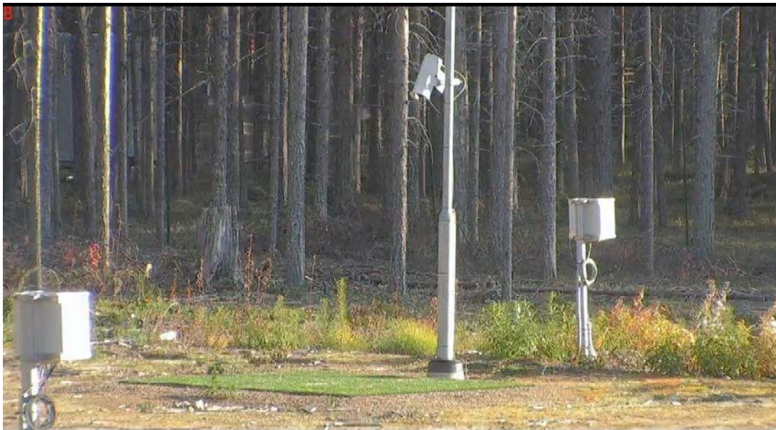
Figure 4.86. The SHM30 and artificial turf target during the snow free period at Sodankylä.
