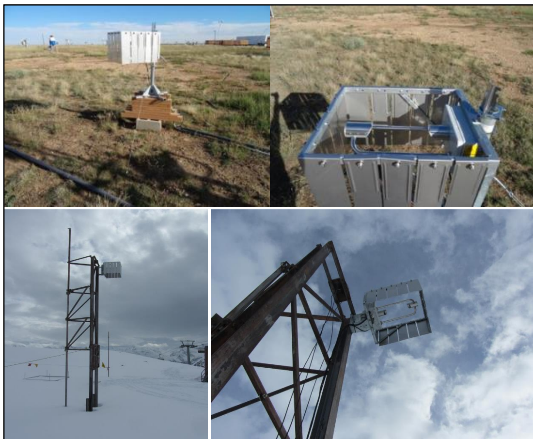
Figure 1: Thies LPM at Marshall (up) and at Weissfluhjoch (bottom) test sites. In both sites, the instrument was installed with a shield provided by the manufacturer.
