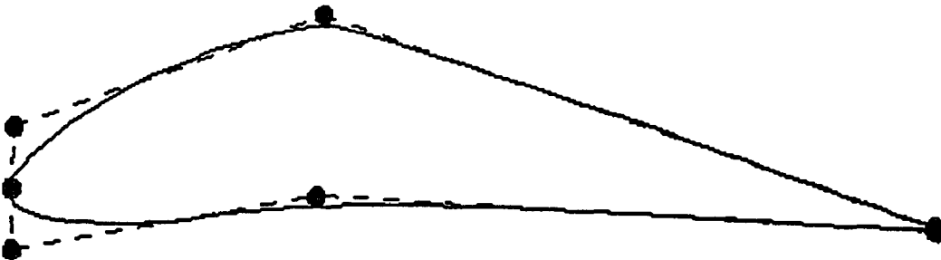
Fig. 2.3 Effect of increasing the weight of control point.
