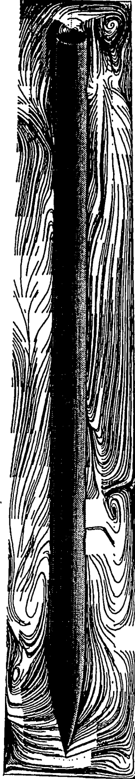
Fig. 4.26 (a) Instantaneous velocity vector (b) Instantaneous streamlines on the symmetry plane of cavity for Case 5.
