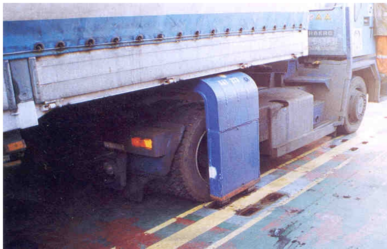
Photograph 7: The SAT lashing system
