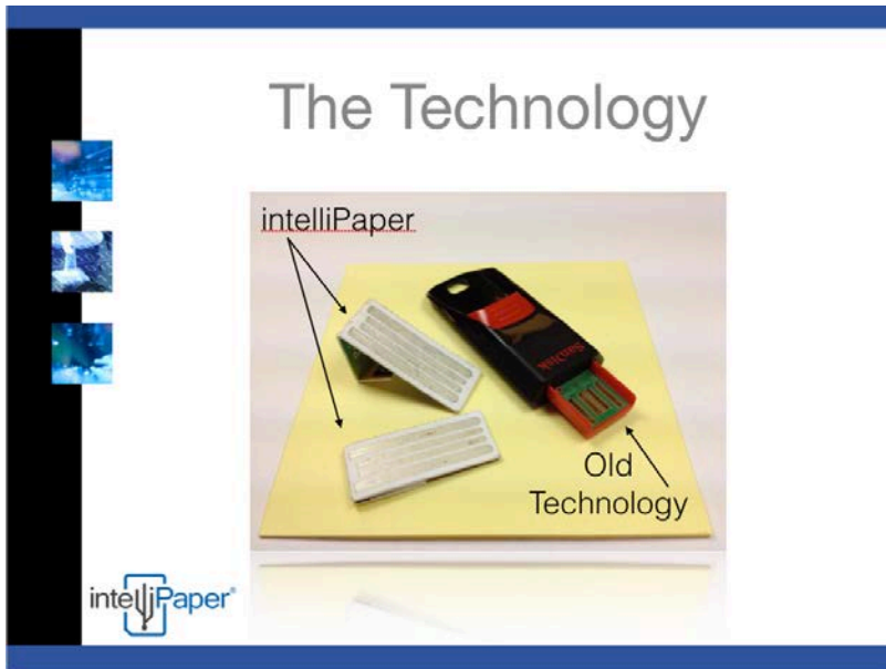
Figure 11. intelliPaper USB design contrasted with the traditional USB technology. (Source: intelliPaper PowerPoint presentation.) Used with permission.
