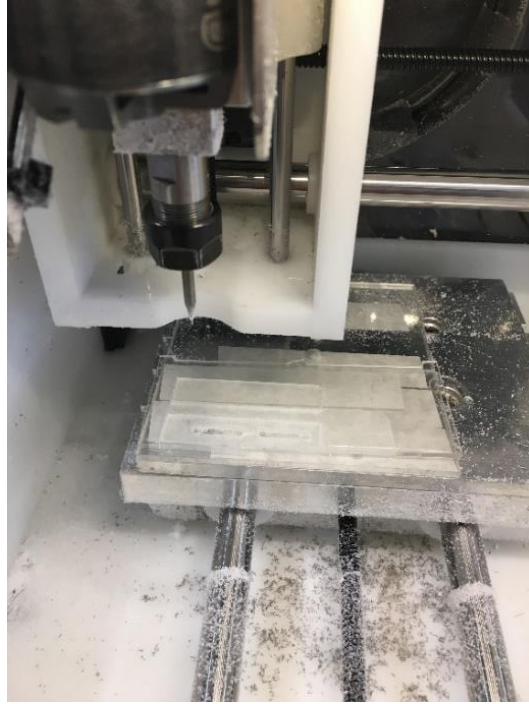
Fig. 3. 11 Machining the microchannel on a PMMA sheet
