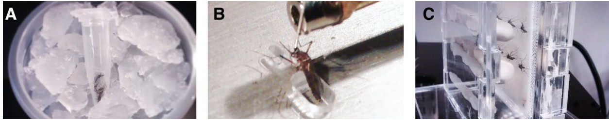
Figure 2.2 Magnetically tethering mosquitoes. (A) Mosquitoes are tethered by anesthetizing on ice. (B) After anesthesia, mosquitoes are transferred to a chill table with forceps. With a micromanipulator and UV-curing glue, a steel pin is glued to the head such that the proboscis points -30 - 45^\circ below horizontal. (C) Mosquitoes are then allowed in a humid enclosure with their legs resting on mesh for at least 1 hour before testing.
