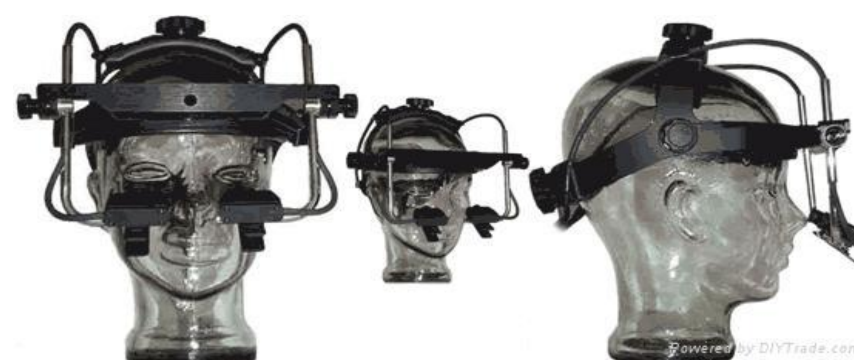
Figure 4. EyeLink II Eye-Tracker
