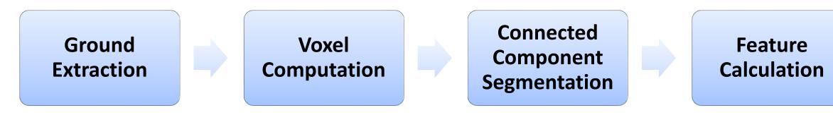
The object space is considered and split into local subsections where a RANSAC based ground estimation is used to estimate the local ground plane. Once the ground points have been identified, the object points are split into a voxelized grid, where each element of the grid is represented by the density of points within that cell space. A three dimensional connected component approach is used to segment out individual objects.
