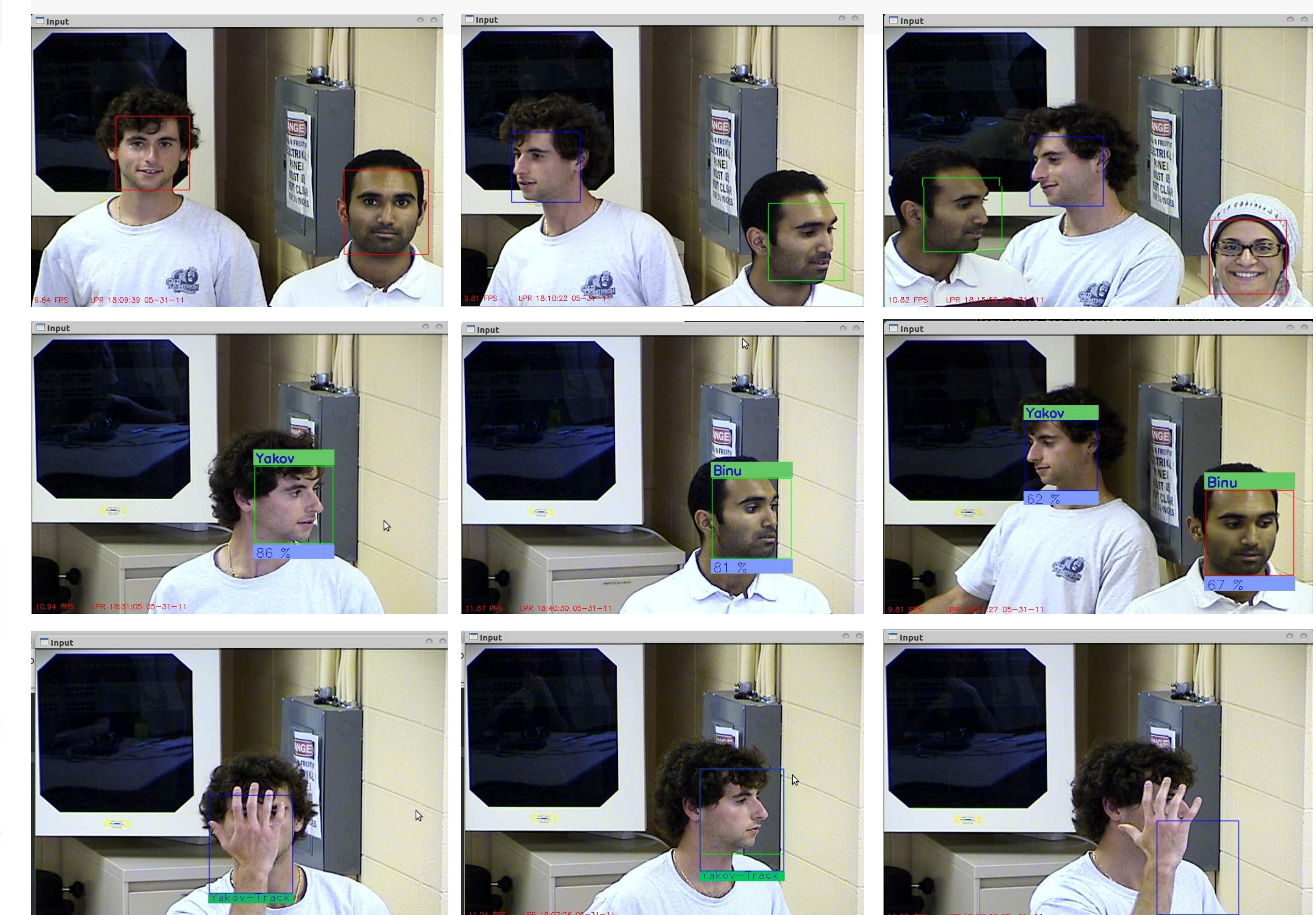
Figure 7- The first line : Face Detection; The second line : Multi-pose Detection and Recognition; The third line : Face Tracking
