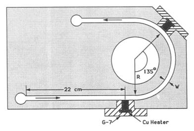
FIGURE 1. Straight and Curved Channel Test Section (R = 2.54 cm, W = 0.32 cm).
