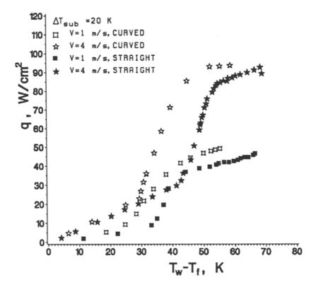
FIGURE 2. Velocity and Geometry Dependence of Nucleate Boiling.
