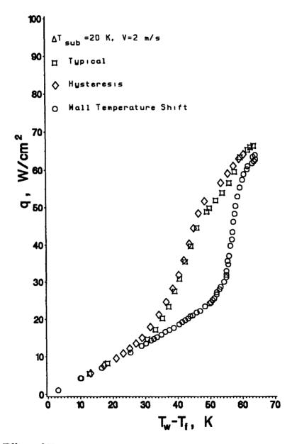
FIGURE 3. Effect of Hysteresis and Temperature Shift of Nucleate Boiling Regime.
