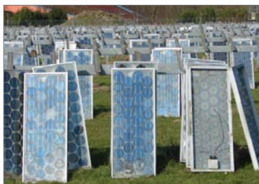
Figure 1-a. Retired PV module in Chevetogn, Belgium after 25+ years of service
