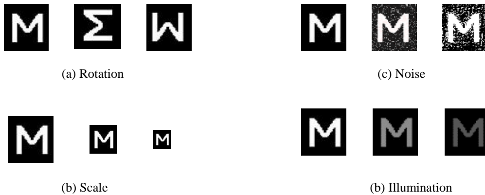
Fig. 1. Illustration of object distortions. First images in (a)-(d) are the reference target image (e.g. letter ‘M’), and the others are the distorted targets.
