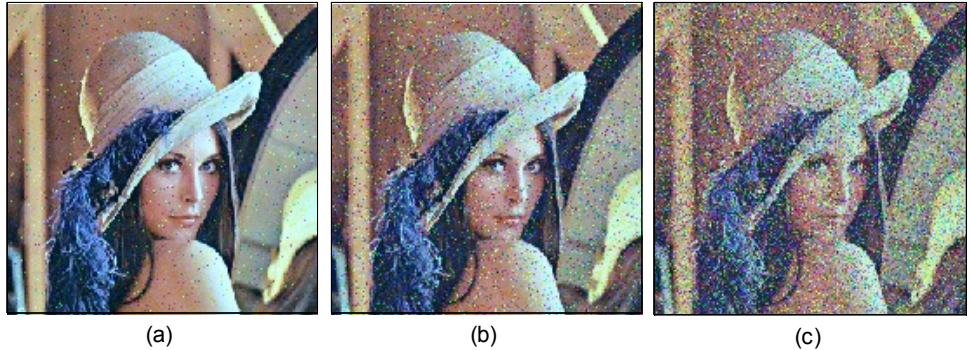
Fig.8. Recovered Lena images with three levels of channel noise power: (a) BER = 0.0073, E_b/N_0= 8 dB, (b) BER =0.0338, E_b/N_0=5 dB, (c) BER =0.1079, E_b/N_0=1 dB.
