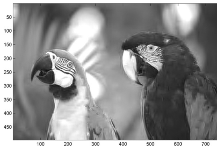
Figure 10 AWF SR with L = 4 is applied on the individually compressed LR images with CR = 8. The optimum SNR of 67.40 is used and \rho = 0.7 .
