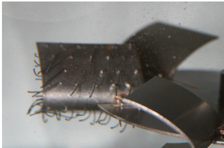
FIGURE 9: Telltales on BT-6 impeller blade.
