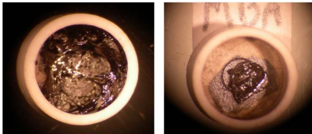
Figure 10. Final chars for TPU + compound 11 (left) and TPU + compound 4 (right).
