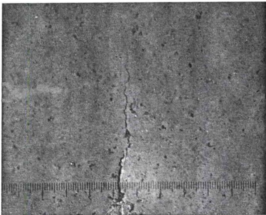
Figure 27: Photo-micrograph of top crack at 1000x. One minor division equals one micron.
