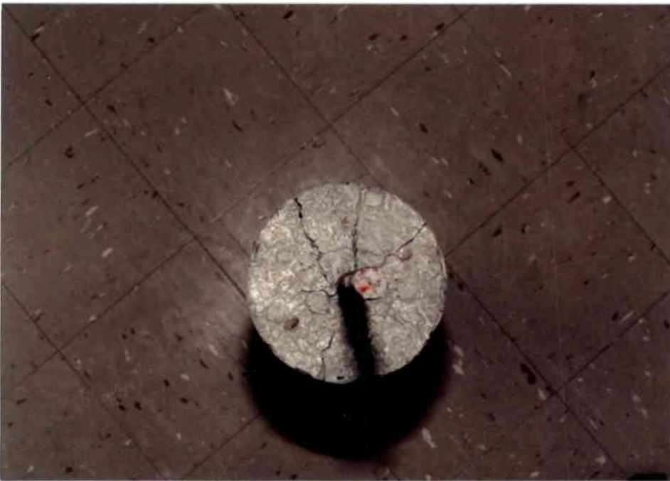
Figure 20. Longitudinal Cracks in a Cylinder. (Top View)
