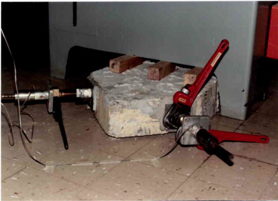
Figure 23. Two-Way Test Set-up. (Side View)
