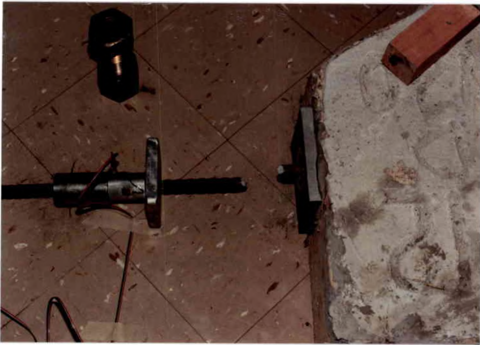
Figure 27. Bar Rupture. (Top View)
