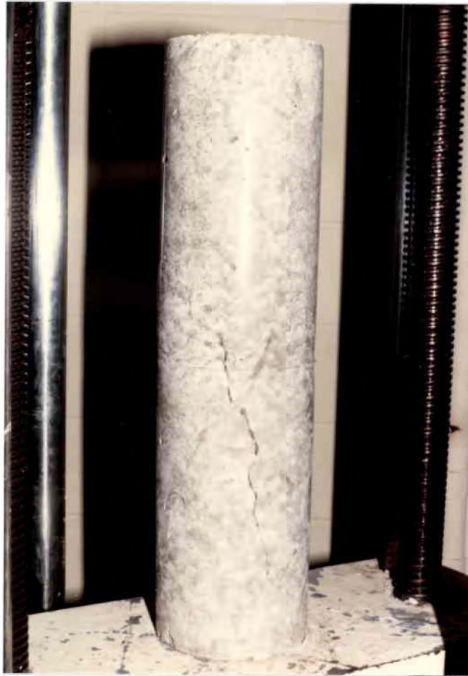
Figure 19. Longitudinal Cracks in a Cylinder Specimen. (Profile)
