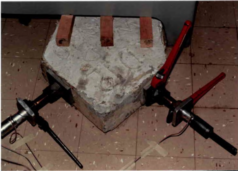
Figure 24. Two-Way Test Set-up. (Top View)
