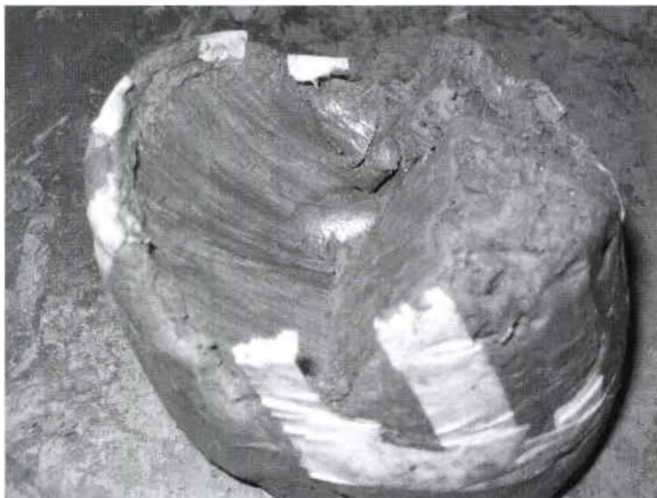
Figure 38 - Failure Surface within Shear-Banded Triaxial Specimen
