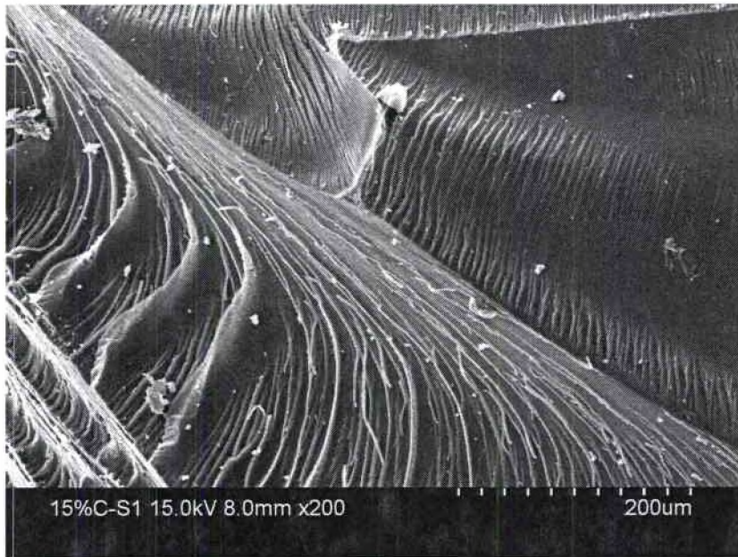
Fig. D.1: 15% Chem-stage fracture surface at 200X magnification.
