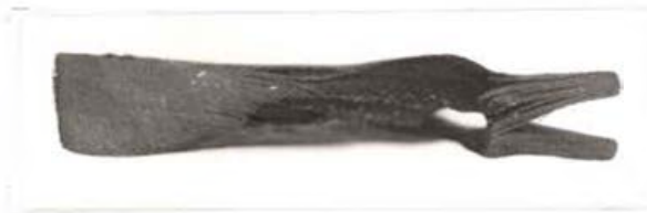
Figure 19. Post Test Photographs of Carbon Phenolic Showing the Effects of Thermal Environment.
