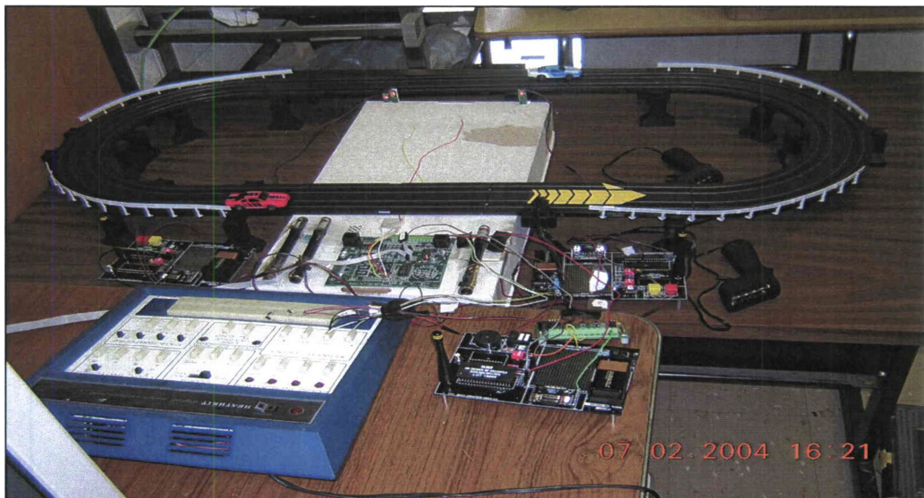
Figure 7: Current transmission-based laser sensor system, as developed in the laboratory.
