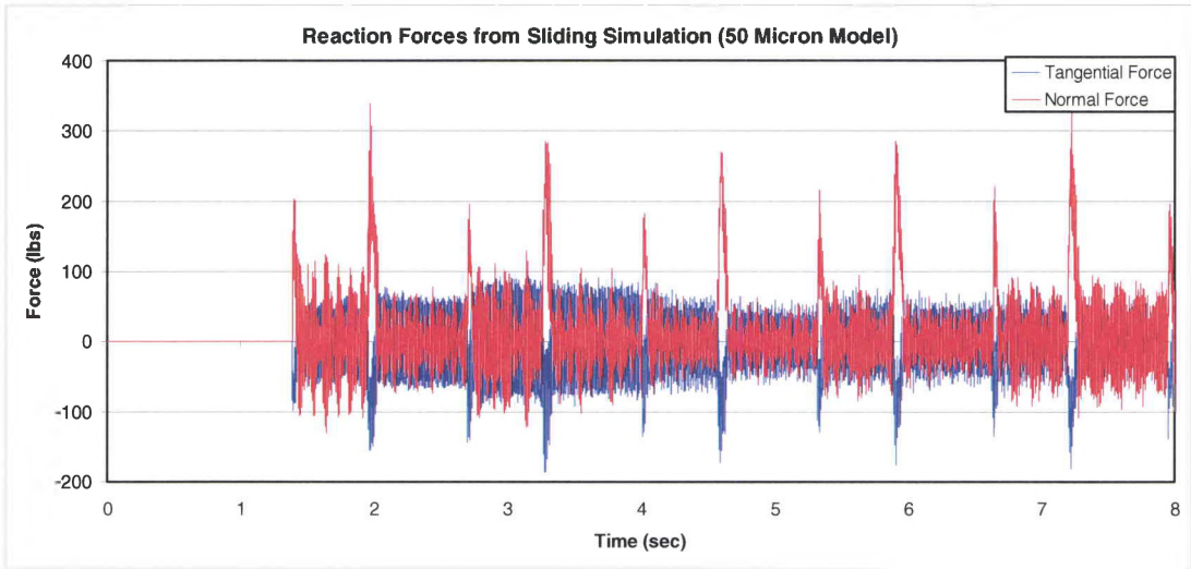
Figure 21: Force resultant from model 1 (50 \mu\text{m} ) sliding simulation
